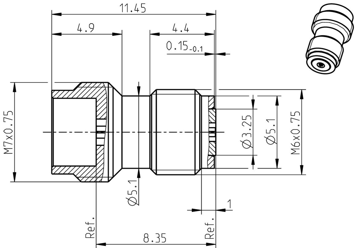
for glass-bead of 0.24mm pin diameter.
