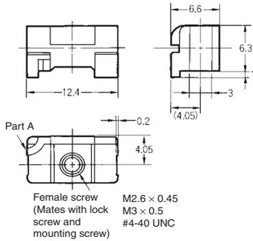
**Note:** When using a Dust Cover, secure the holding ring at part A.
