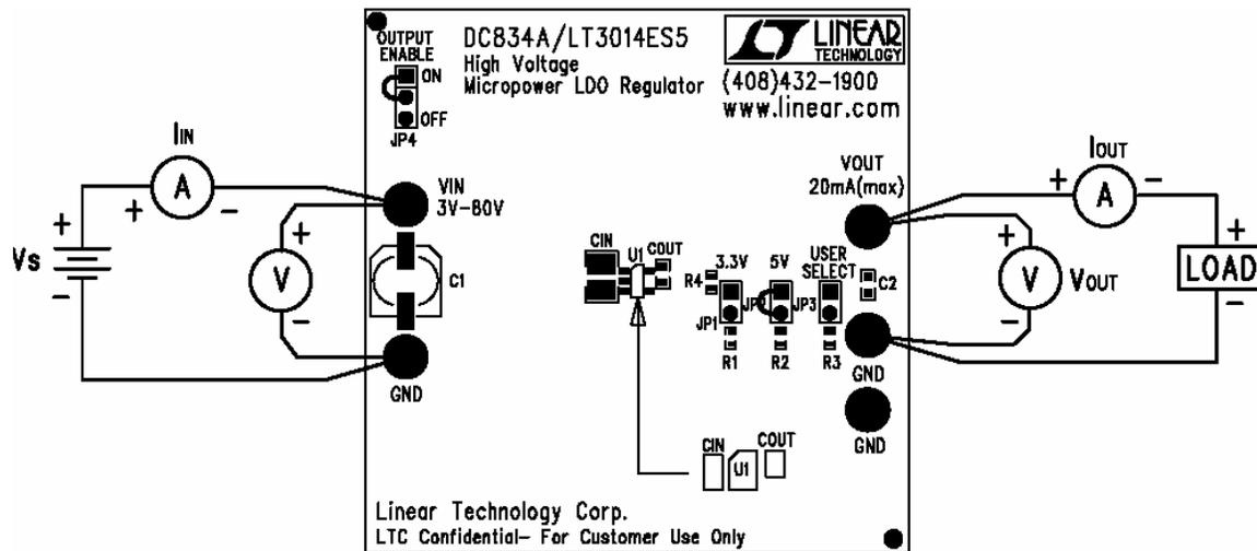
Figure1. Proper Measurement Equipment Setup
