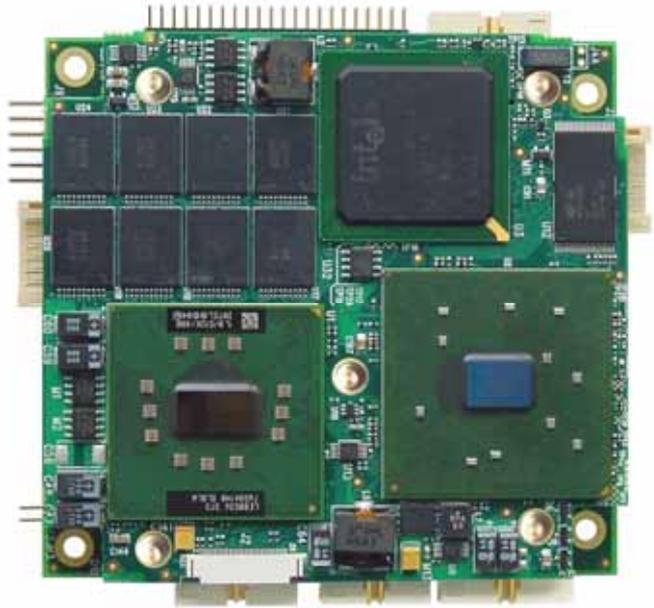
The CPU-1482 is an embedded RoHS compliant board based on two modules: a mezzanine CPU module combined with a PC/104-Plus form factor carrier.
