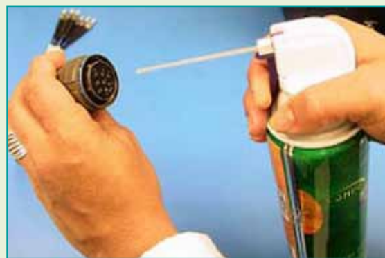
Compressed-air cleaning of a connector face, and swab cleaning of ferrule/fiber end of socket termini
