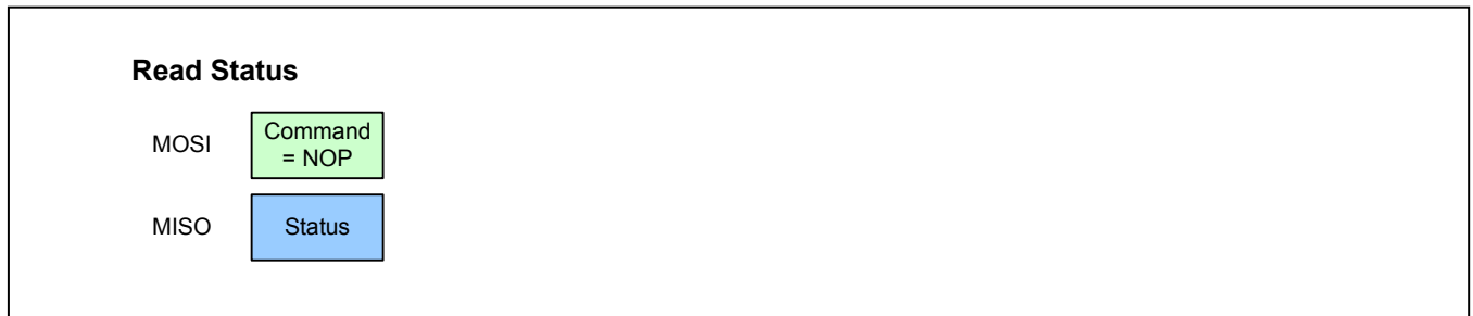
Figure 3.6 SPI Read Status.
