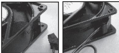
FANS WITH TERMINALS MAKE CONNECTING AND DISCONNECTING POWER A BREEZE.
