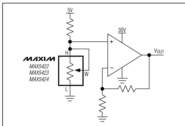
Figure 4. Positive LCD-Bias Control Using a Variable Resistor
