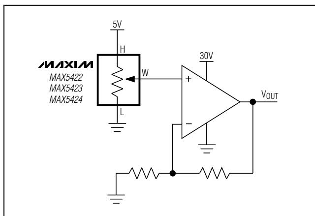
Figure 3. Positive LCD-Bias Control Using a Voltage-Divider
