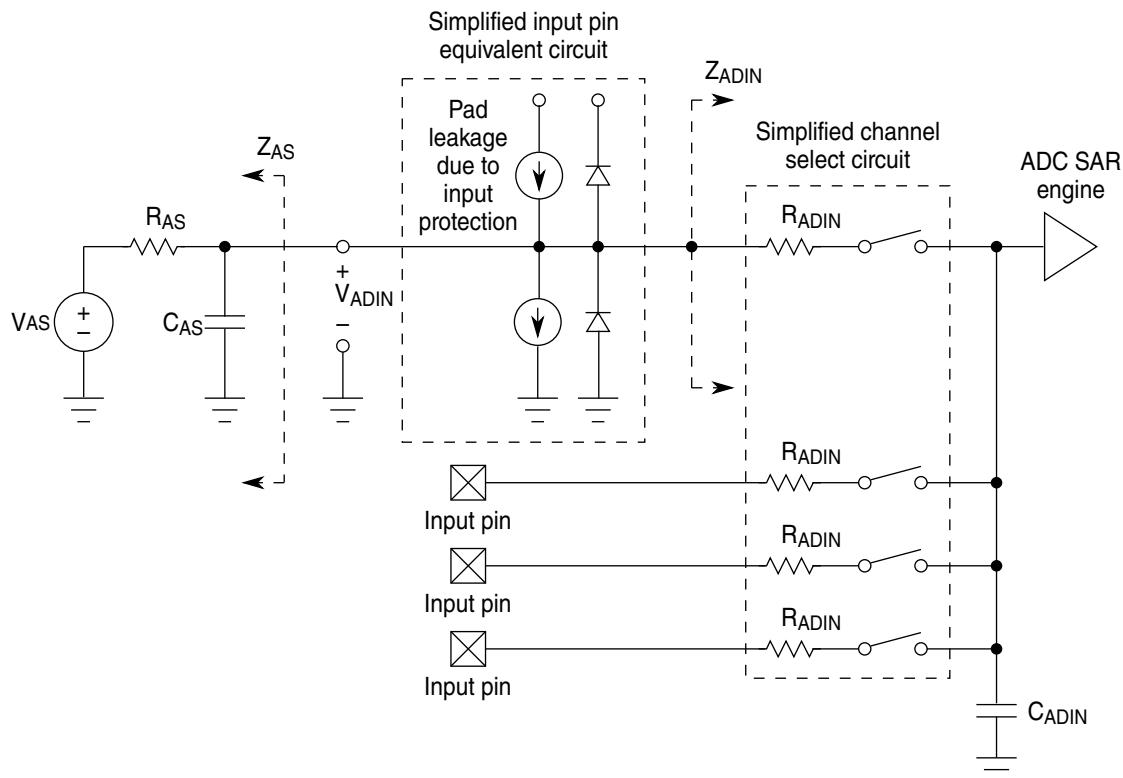
**Figure 5. 12-bit ADC Input Impedance Equivalency Diagram**
