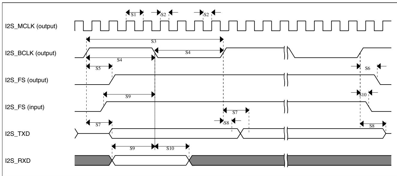
**Figure 28. SAI Timing — Master Modes****Table 47. Slave Mode SAI Timing**
