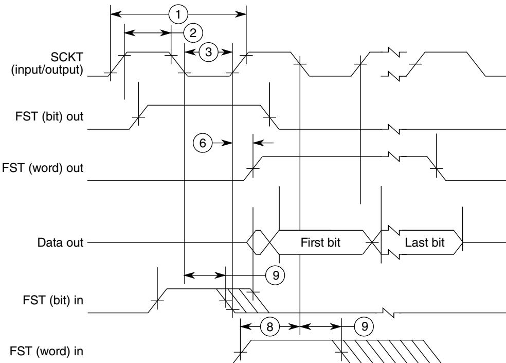
**Figure 24. ESDAI Transmitter Timing**
