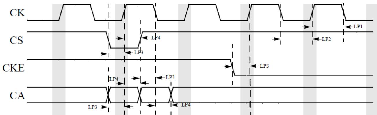
**Figure 44. LPDDR2 Command and Address timing parameter**
