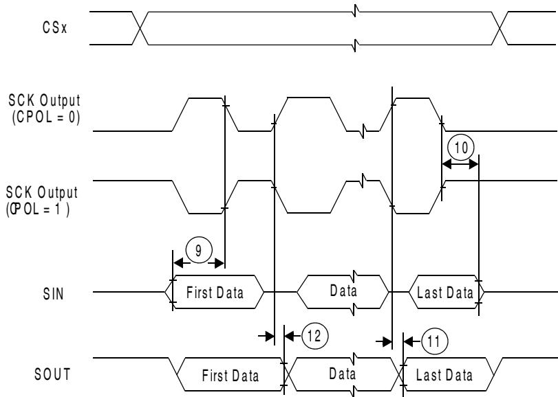
**Figure 49. DSPI classic SPI timing master, CPHA=1**
