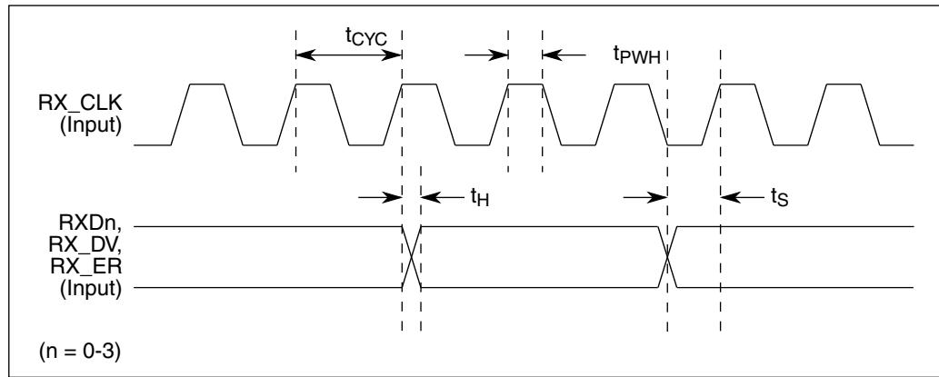
**Figure 22. MII receive signal timing diagram****Table 42. Receive signal timing for MII interfaces**
