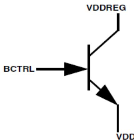
**Figure 3. External NPN Ballast connections****Table 6. BCTRL OUTPUT specification**
