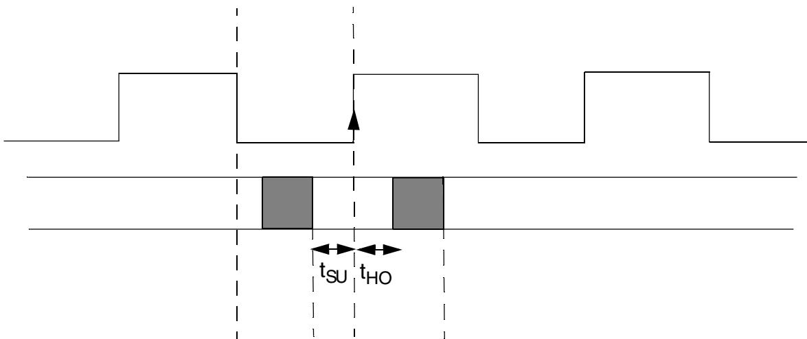
**Figure 18. VIU Timing Parameters****Table 38. VIU Timing Parameters**
