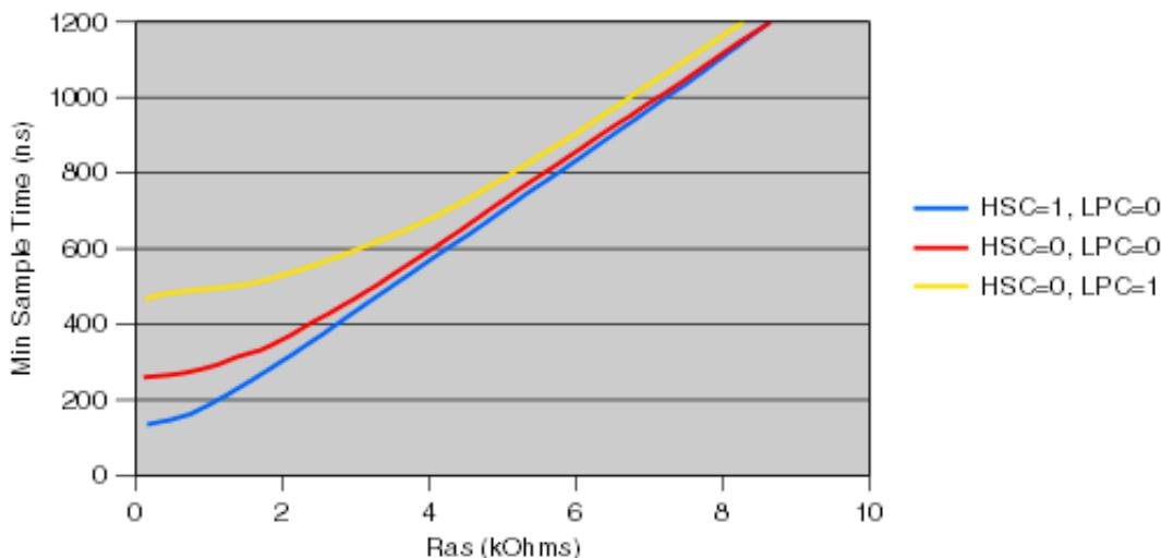
**Figure 8. Minimum Sample Time Vs Ras (Cas = 10pF)**
