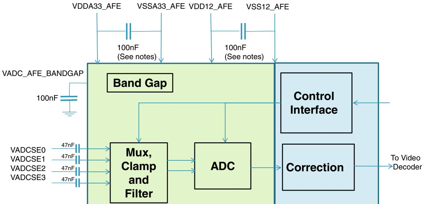
**Figure 12. VideoADC supply scheme**
