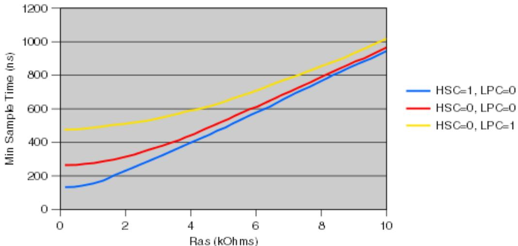
**Figure 7. Minimum Sample Time Vs Ras (Cas = 5pF)**
