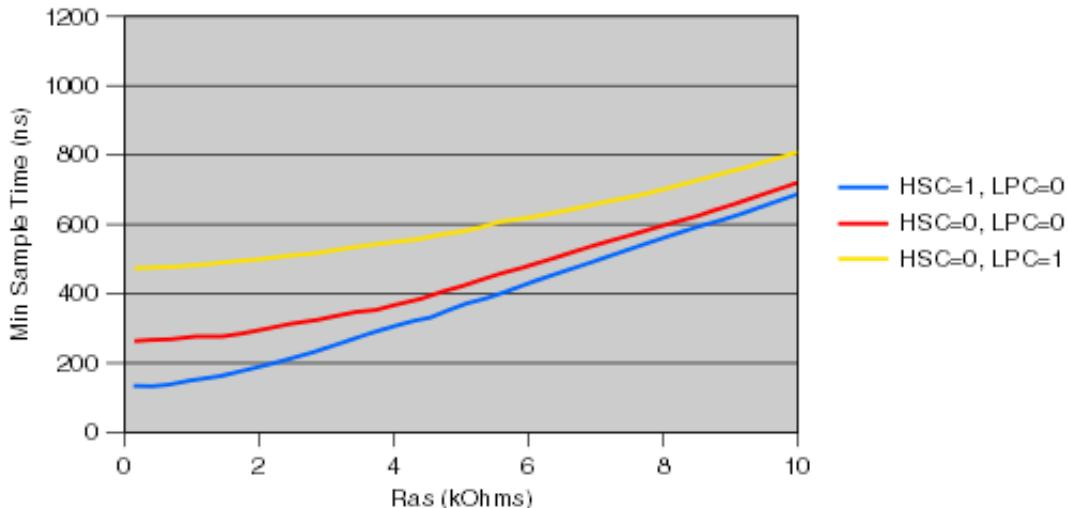
**Figure 6. Minimum Sample Time Vs Ras (Cas = 2pF)**
