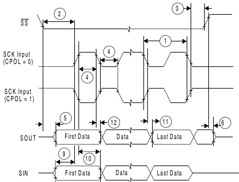
**Figure 50. DSPI classic SPI timing slave, CPHA=0**
