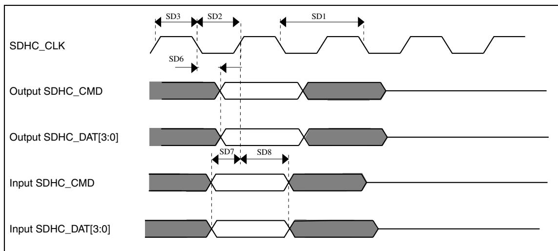
**Figure 53. SDHC timing**
