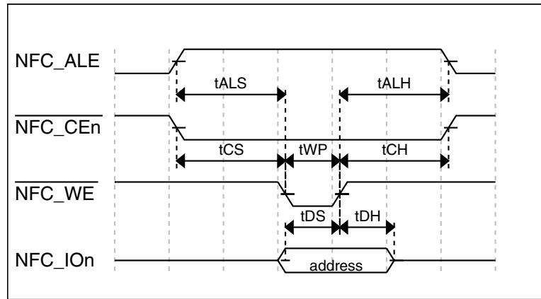
**Figure 35. Address latch cycle timing**
