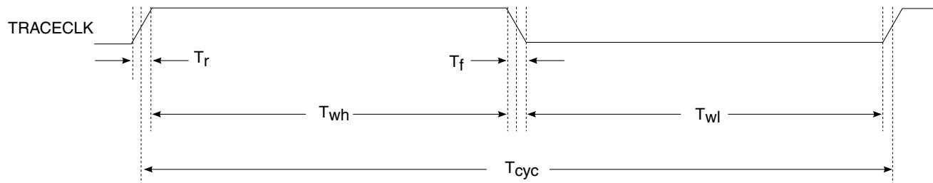
Figure 57. TRACE\_CLKOUT specifications
