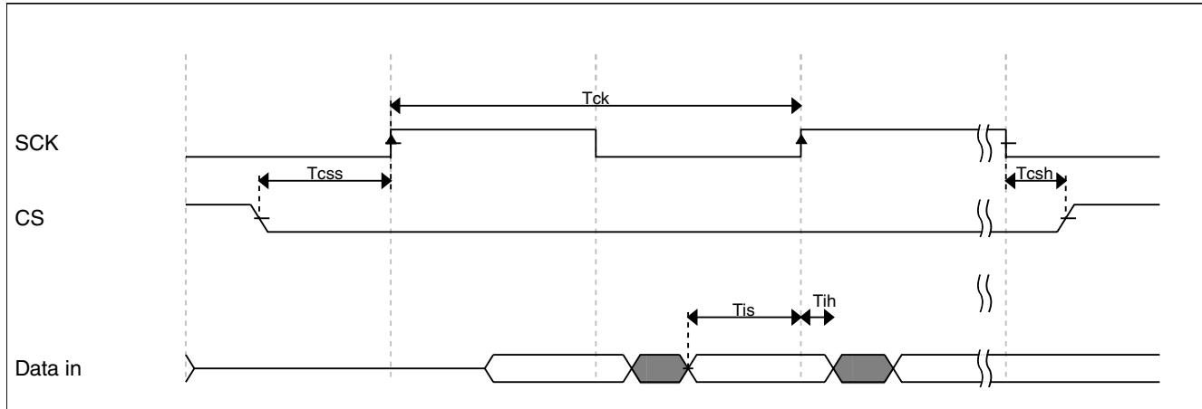
**Figure 32. QuadSPI Input/Read timing (DDR mode)****NOTE**
