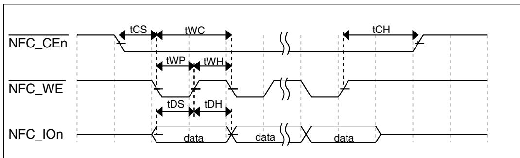
**Figure 36. Write data latch cycle timing**
