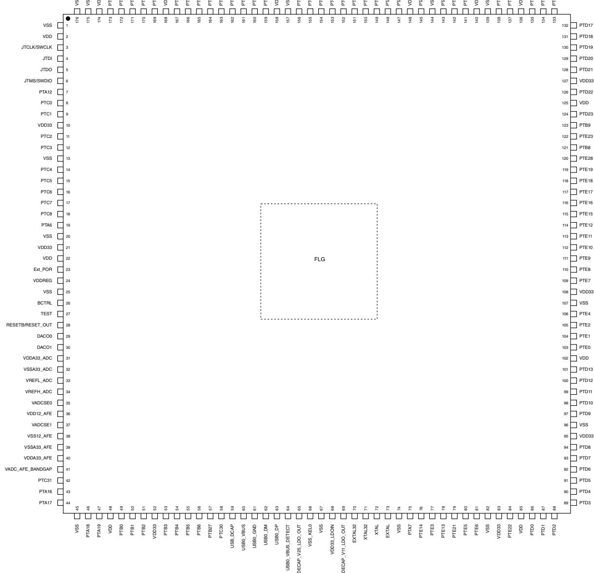
**Figure 59. 176 LQFP Pinout Diagram**
