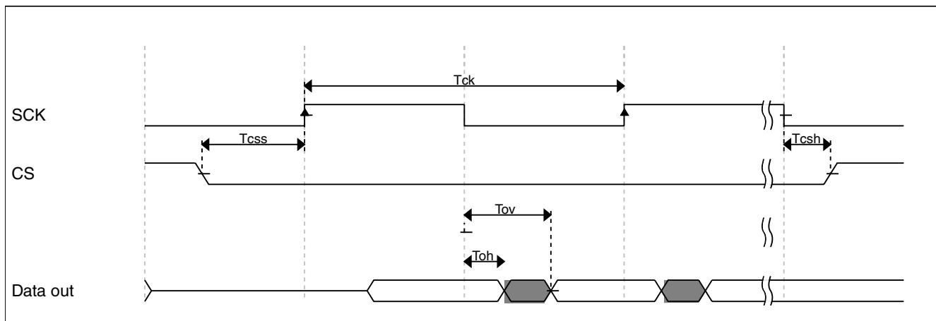
**Figure 33. QuadSPI Output/Write timing (DDR mode)****Table 51. QuadSPI Output/Write timing (DDR mode)**
