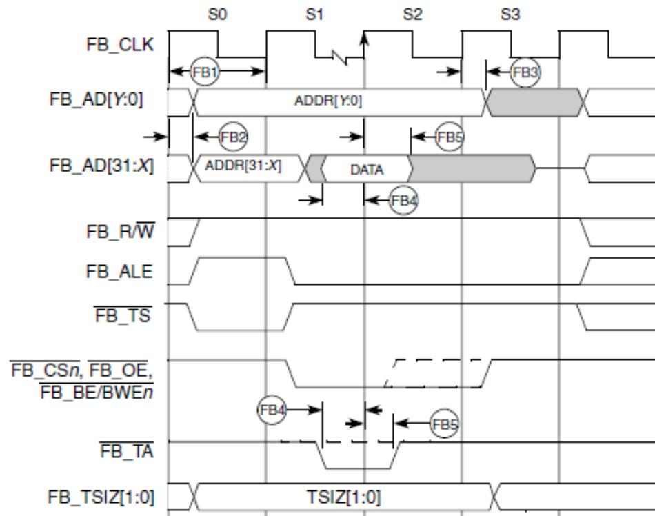
**Figure 39. FlexBus read timing**
