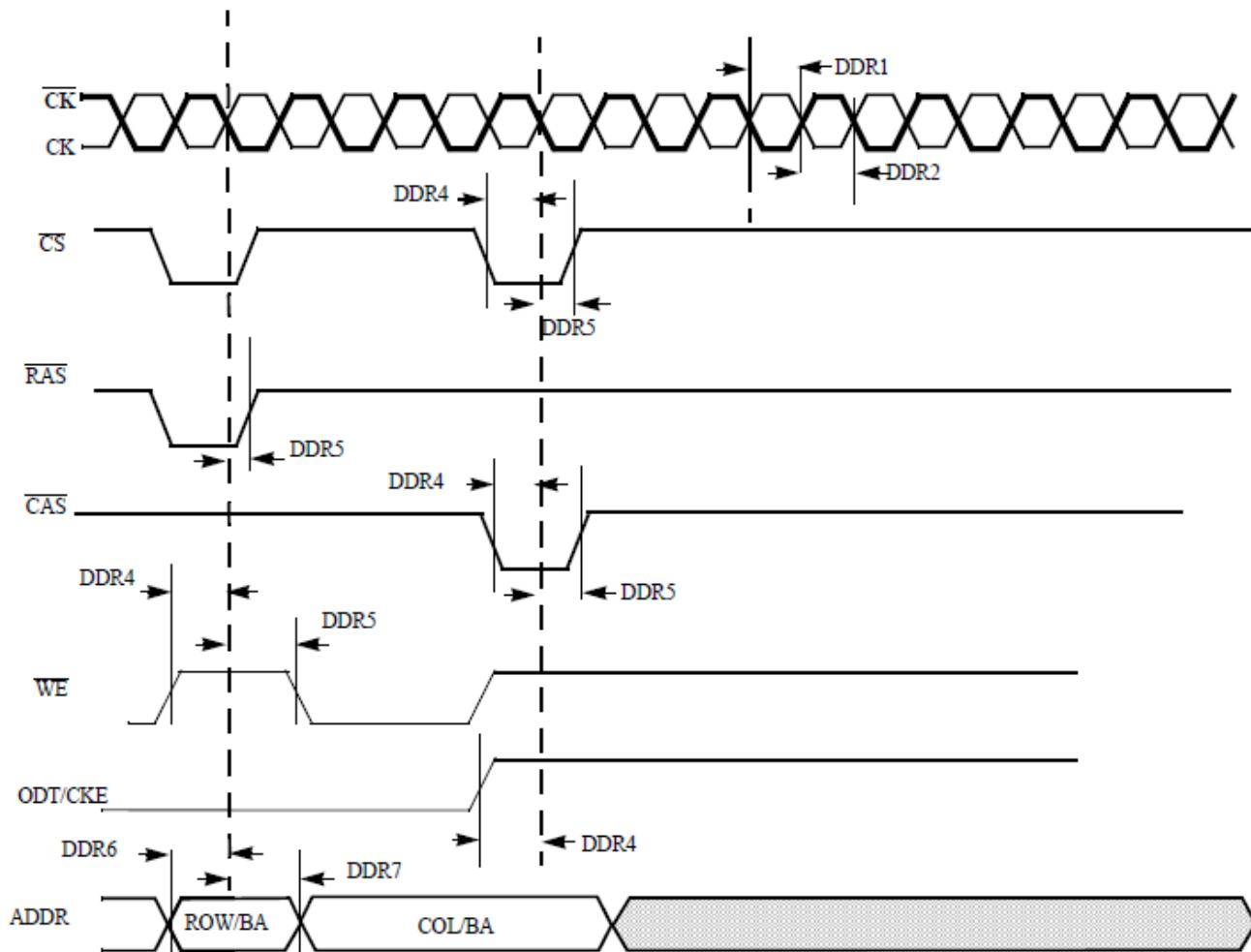
Figure 41. DDR3 Command and Address Timing Parameters
