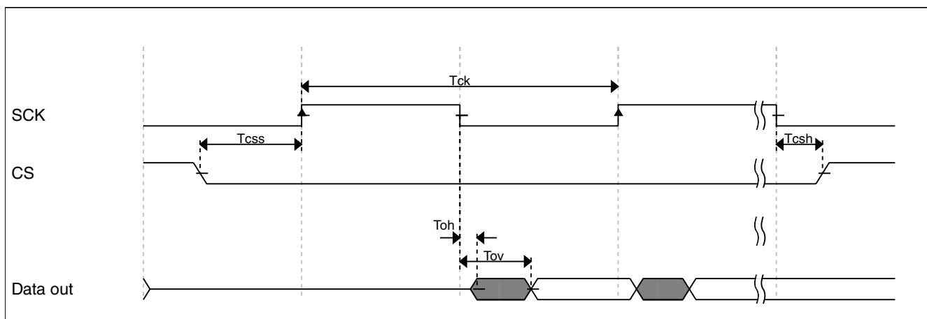
**Figure 31. QuadSPI Output/Write timing (SDR mode)****Table 49. QuadSPI Output/Write timing (SDR mode)**
