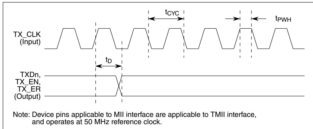
**Figure 23. MII transmit signal timing diagram****Table 43. Transmit signal timing for MII interfaces**
