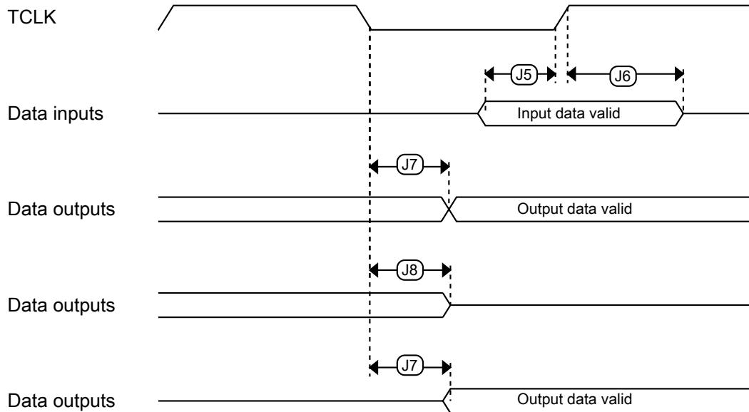
Figure 55. Boundary scan (JTAG) timing
