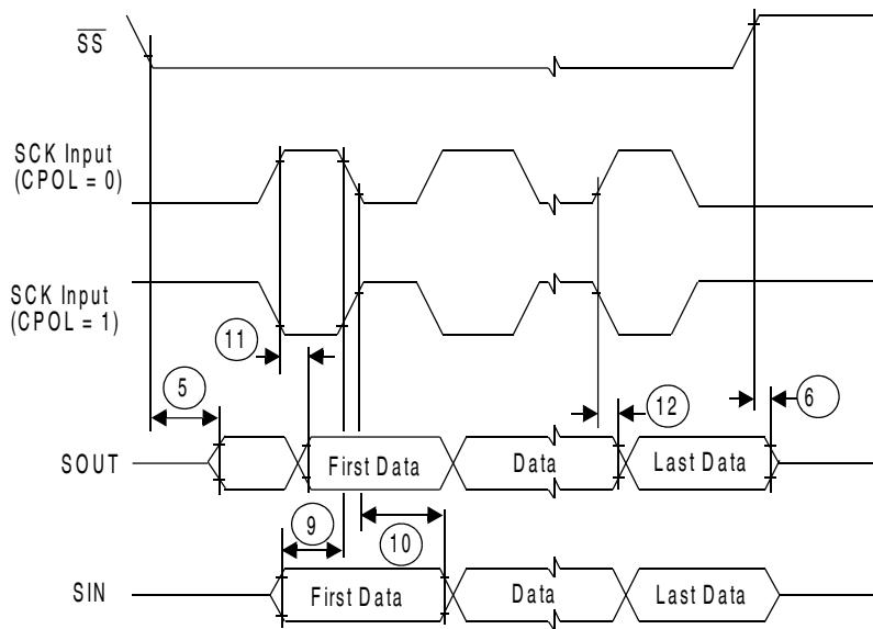
Figure 51. DSPI classic SPI timing slave, CPHA=1
