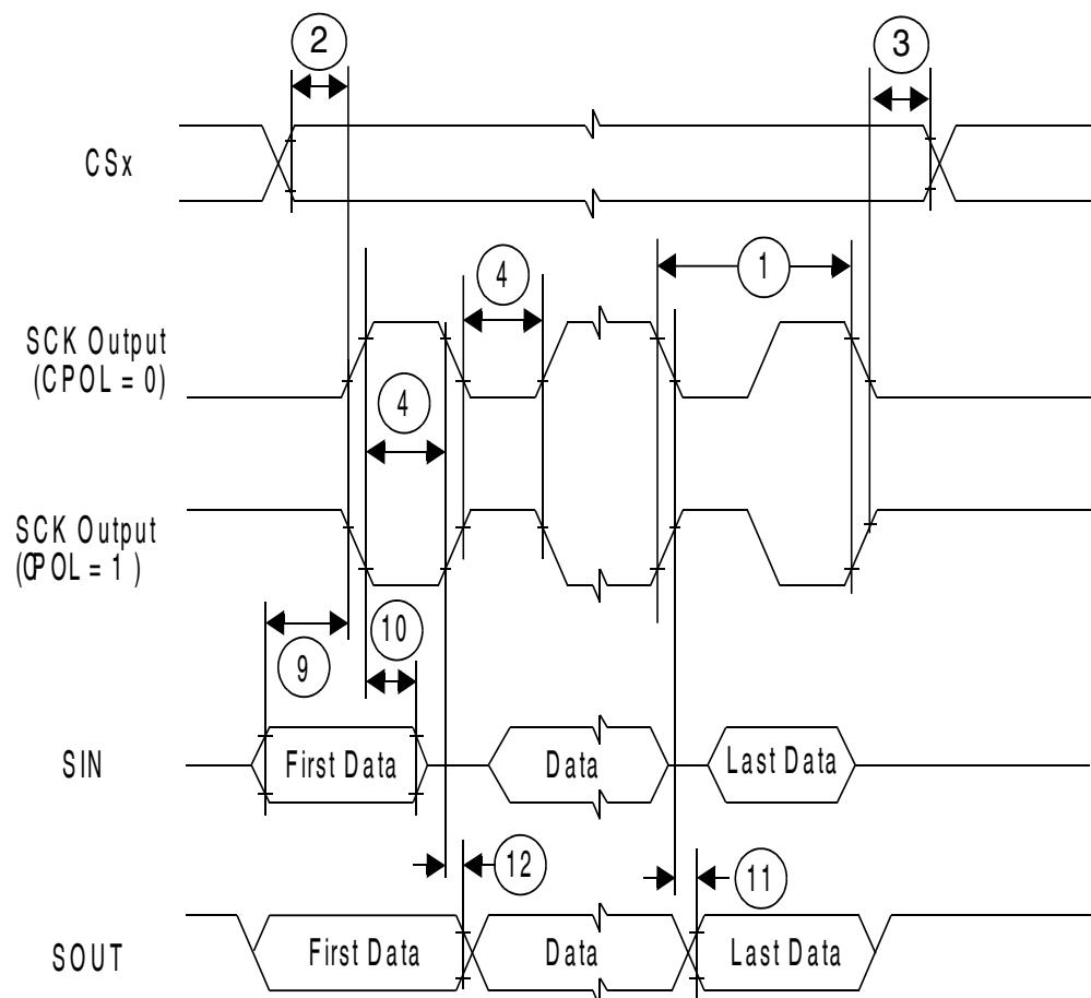
**Figure 48. DSPI classic SPI timing master, CPHA=0**
