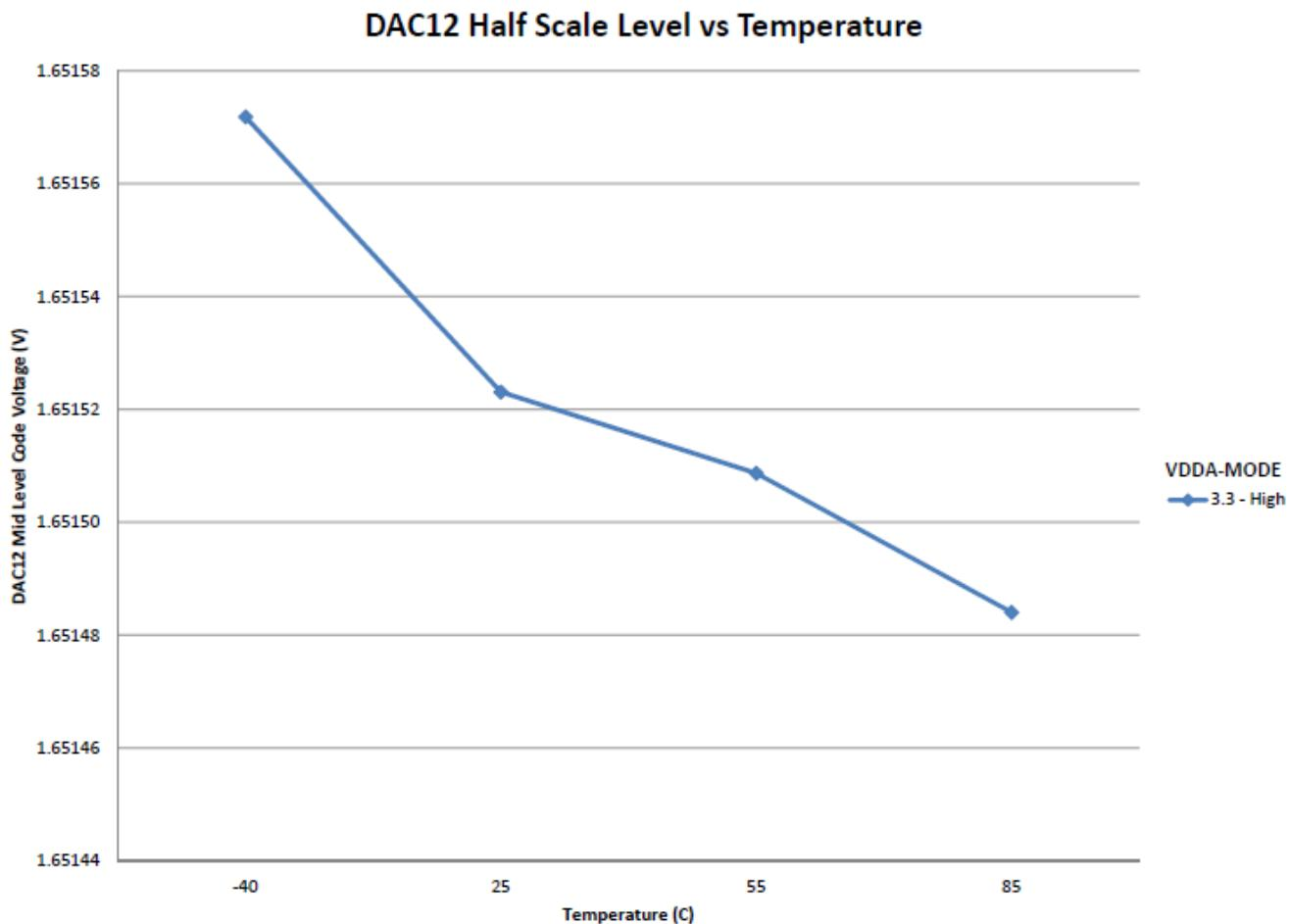
**Figure 11. Offset at half scale vs. temperature**
