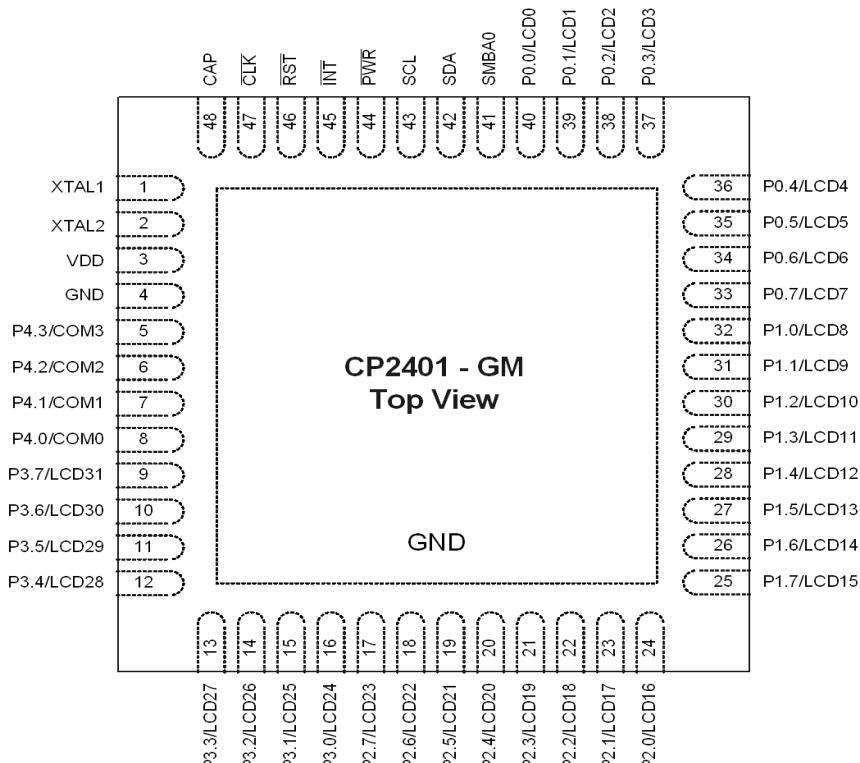
**Figure 4.4. CP2401-GM Pinout (SMBus/I<sup>2</sup>C Interface)**
