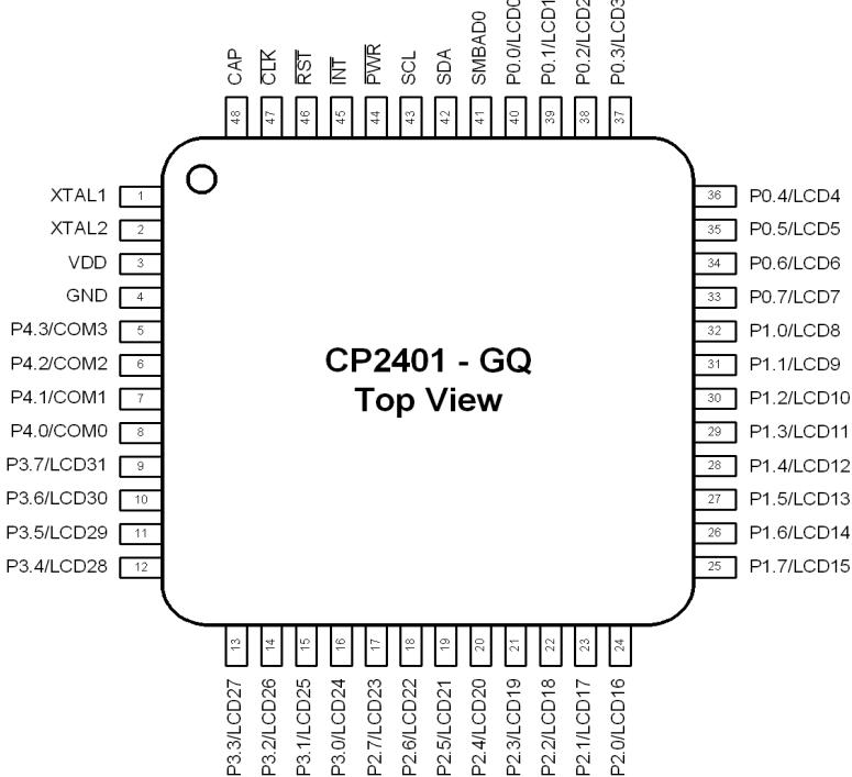
**Figure 4.2. CP2401-GQ Pinout (SMBus/I<sup>2</sup>C Interface)**
