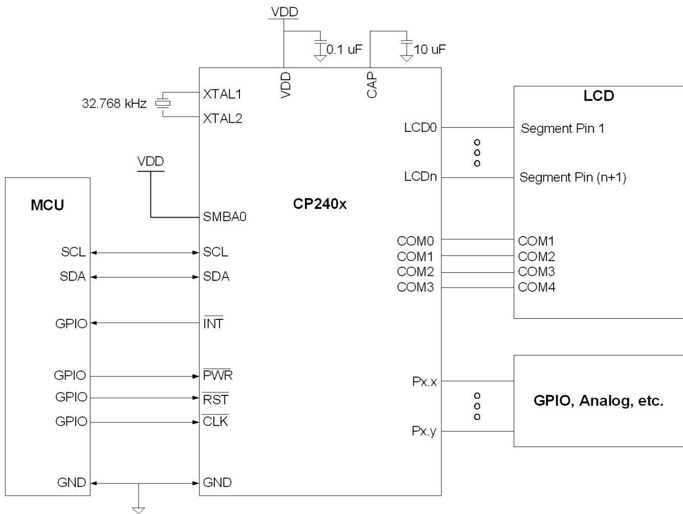
Figure 1.6. Typical Connection Diagram (SMBus/I<sup>2</sup>C Interface)
