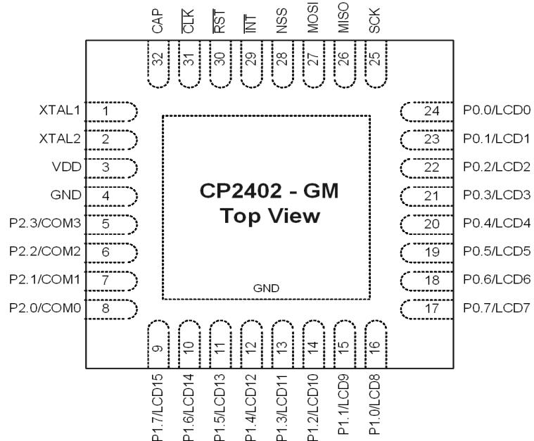
**Figure 4.5. CP2402-GM Pinout (SPI Interface)**
