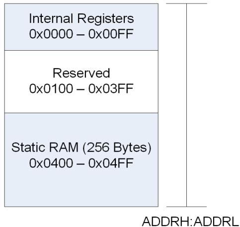
**Figure 6.1. Internal Register and RAM Memory Map**
