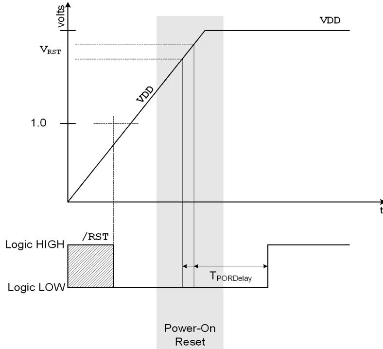
Figure 8.1. Reset Timing
