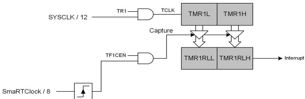
**Figure 13.3. Timer 1 Capture Mode Block Diagram**
