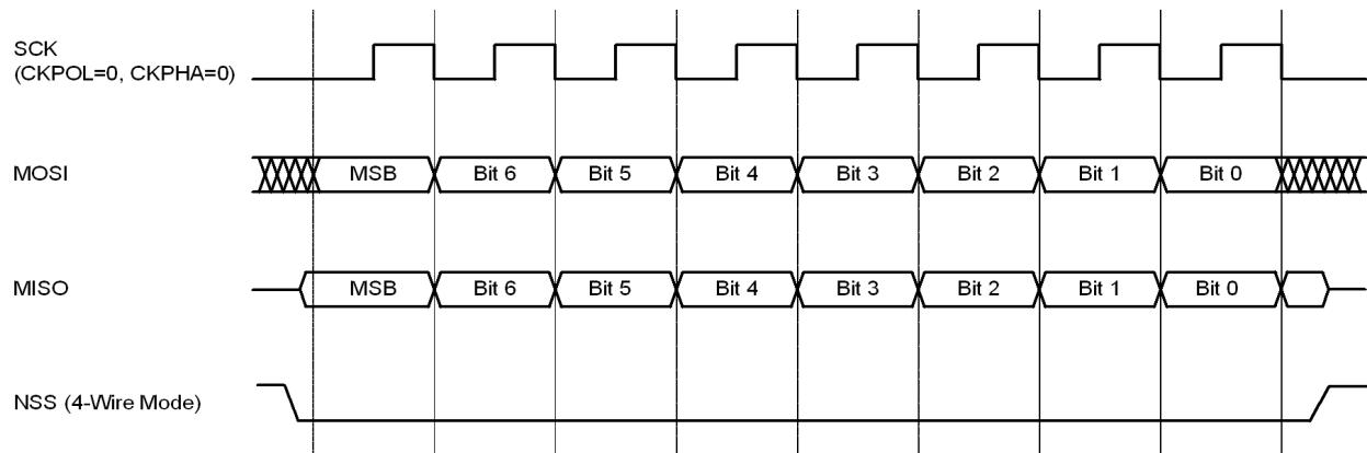
Figure 14.2. Data/Clock Timing
