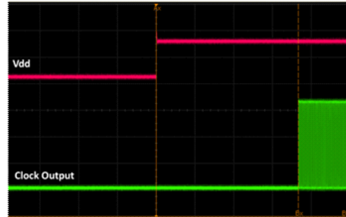
Figure 17. Startup Waveform vs. Vdd
