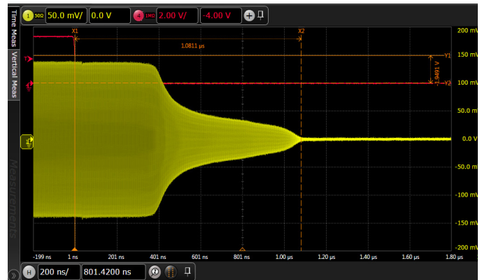
Figure 15. Switching Time [Insertion Loss to Isolation State]
