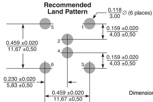
Dimensions are in  $\frac{\text{inches}}{\text{mm}}$
