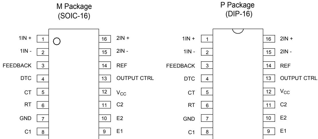
Figure 2. Pin Configuration of AZ7500B (Top View)
