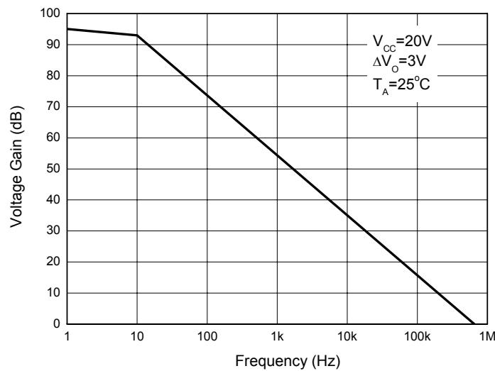
Figure 9. Error Amplifier Small-Signal Voltage Gain vs. Frequency
