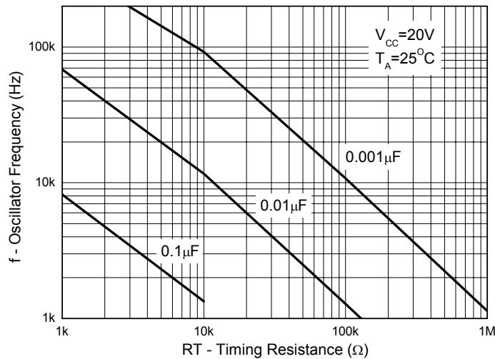
Figure 8. Oscillator Frequency vs. RT and CT
