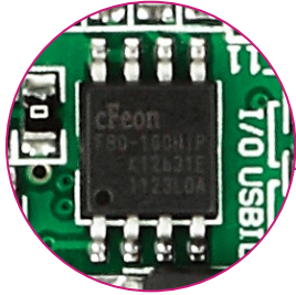
Figure 11-1: Flash memory module
