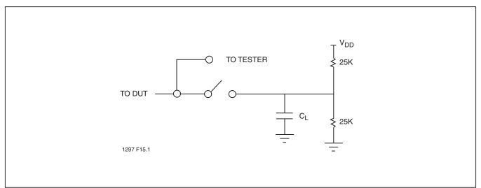
FIGURE 18: A Test Load Example
