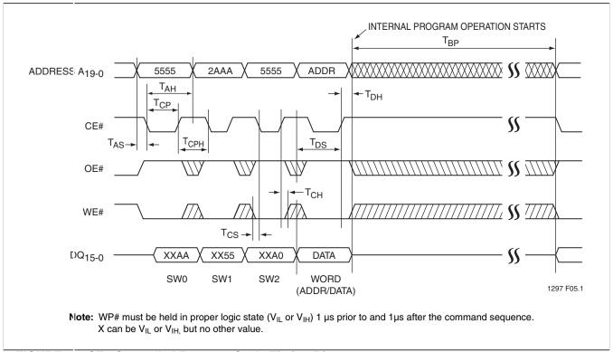
FIGURE 5: CE# Controlled Program Cycle Timing Diagram
