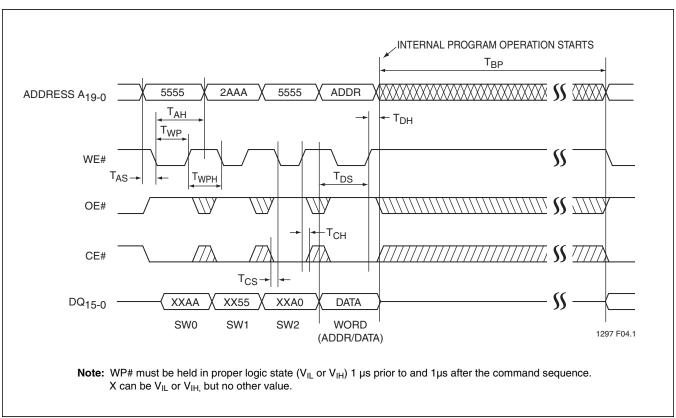
FIGURE 4: WE# Controlled Program Cycle Timing Diagram
