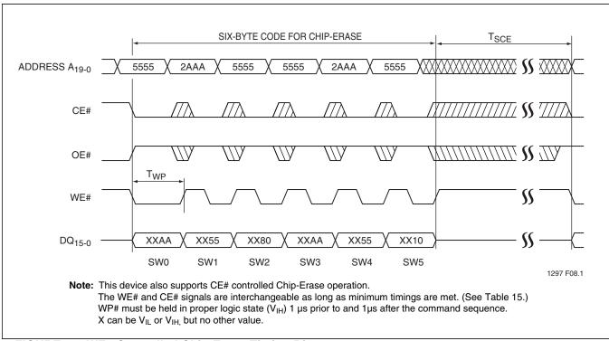
FIGURE 8: WE# Controlled Chip-Erase Timing Diagram
