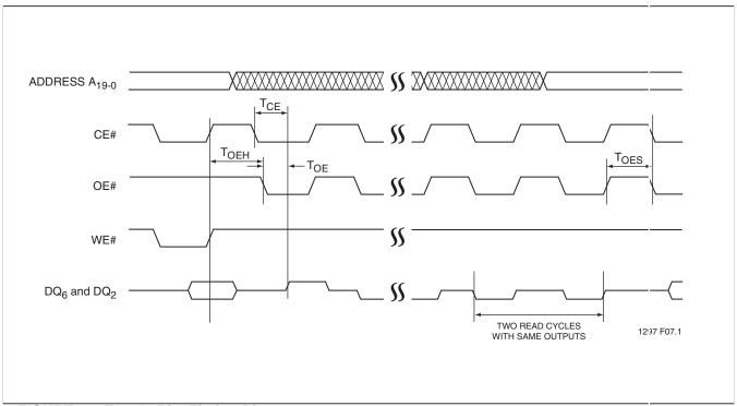
FIGURE 7: Toggle Bits Timing Diagram
