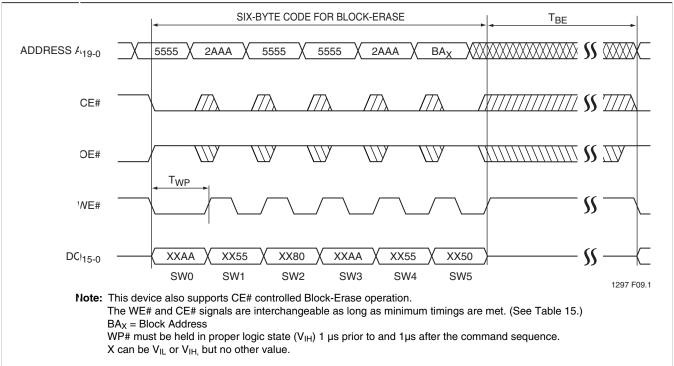
FIGURE 9: WE# Controlled Block-Erase Timing Diagram
