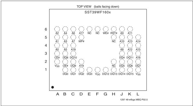
FIGURE 2: Pin assignments for 48-ball WFBGA
