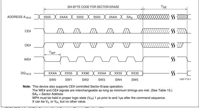
FIGURE 10: WE# Controlled Sector-Erase Timing Diagram
