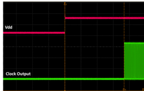
Figure 17. Startup Waveform vs. Vdd
