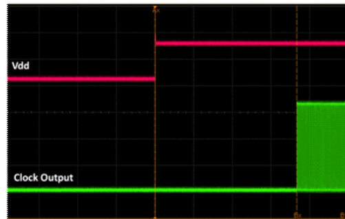
Figure 17. Startup Waveform vs. Vdd
