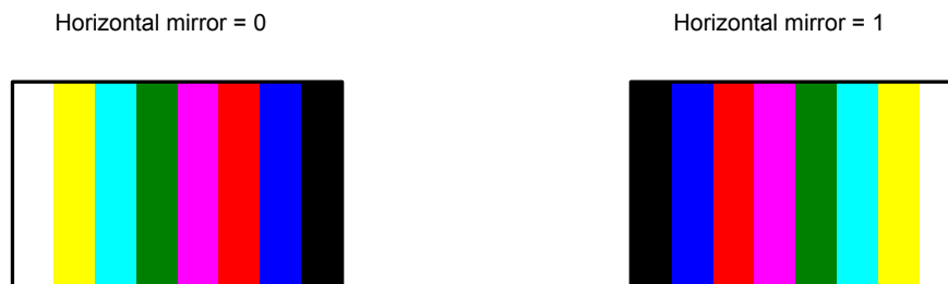
Figure 56: 100% Color Bars Test Pattern
