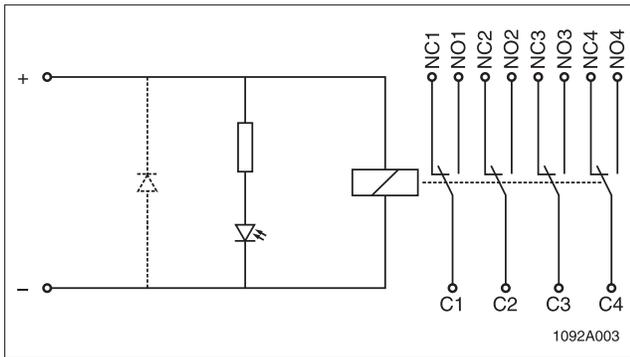
Figure 3. UMK 33 Relay Base Block Diagram
