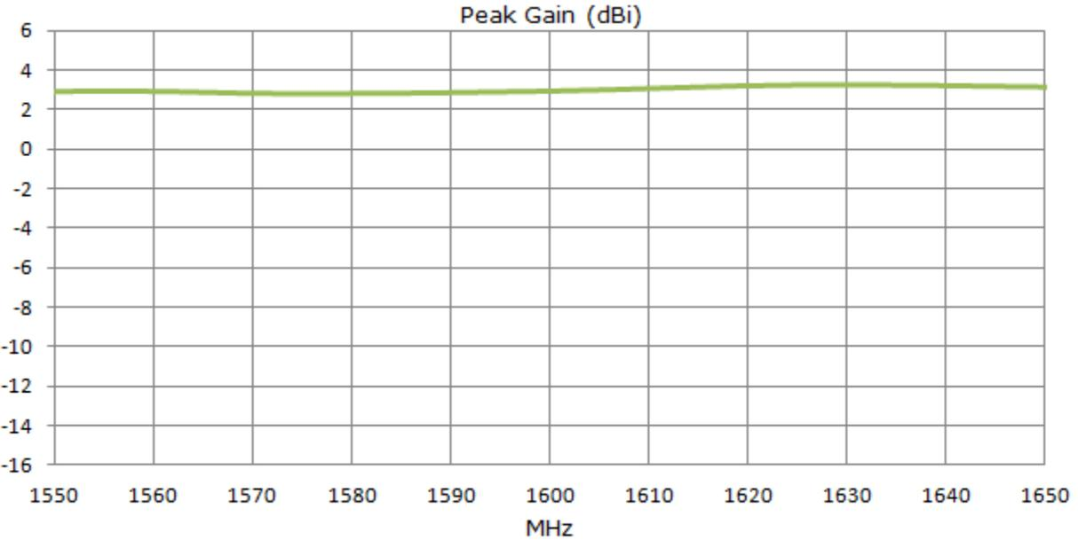
**Figure 5:** Peak Gain of FXP611 GPS/GLONASS/GALILEO/BeiDou Antenna
