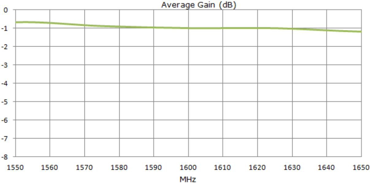
**Figure 6:** Average Gain of FXP611 GPS/GLONASS/GALILEO/BeiDou Antenna
