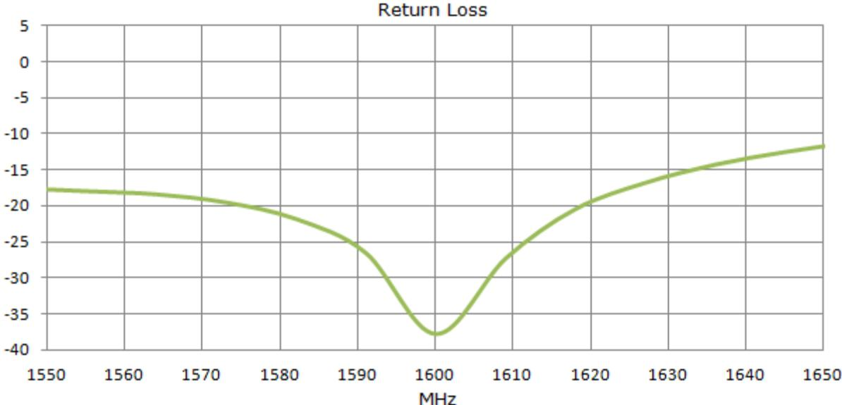
**Figure 2:** Return loss of FXP611 GPS/GLONASS/GALILEO/BeiDou Antenna
