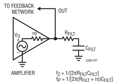
Figure 7. Pole-Zero Introduced by RC Network at Output
