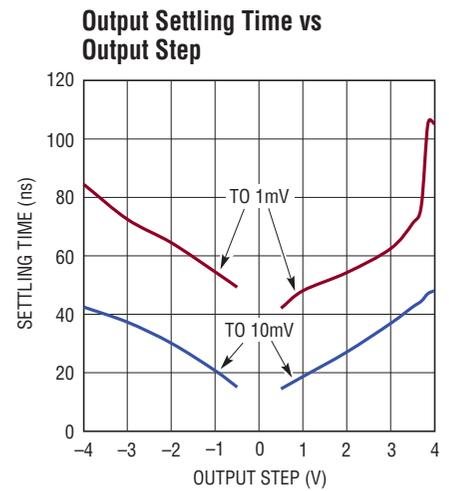
**TYPICAL PERFORMANCE CHARACTERISTICS**  $T_A = 25^\circ\text{C}$ ,  $V_{CC} = V_{DD} = 5\text{V}$ ,  $V_{+IN} = 2\text{V}$ ,  $V_{SHDN} = 5\text{V}$ , see Figure 1 for circuit configuration.
