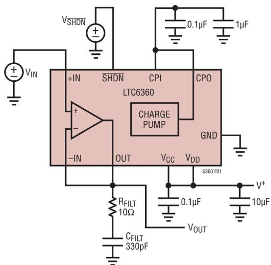
Figure 1. Test Circuit
