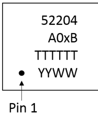
Figure 10.11. Si52204 Top Marking
