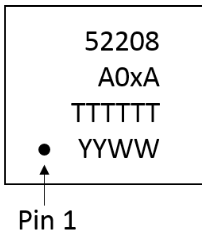
Figure 10.10. Si52208 Top Marking
