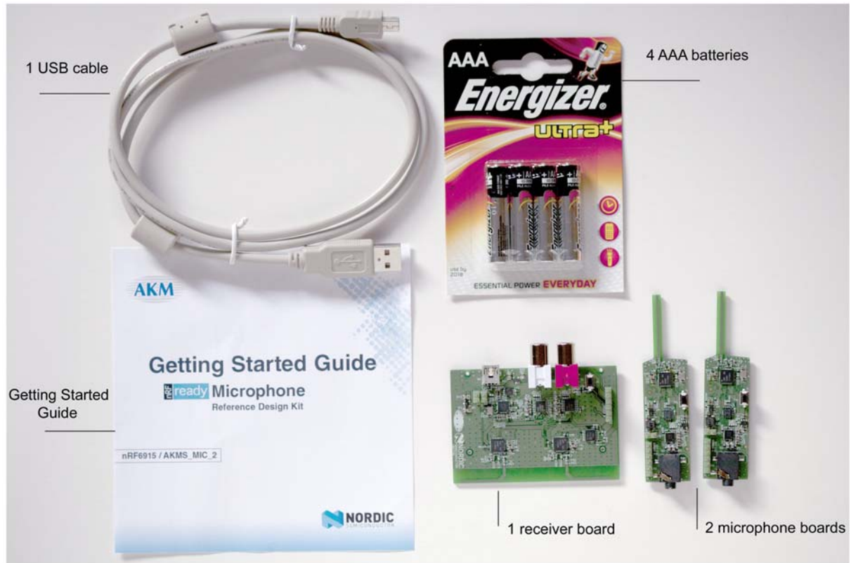
Figure 1. nRFready Microphone Development Kit content
