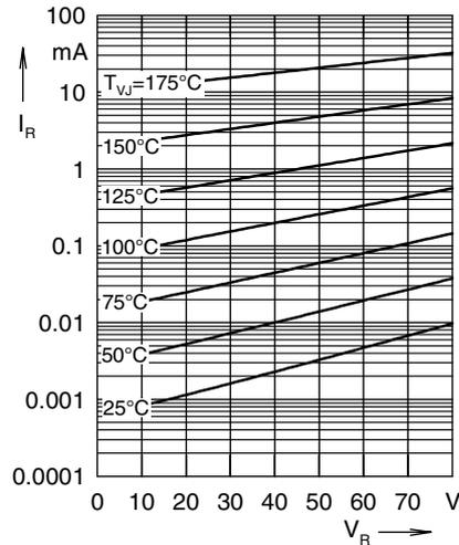
Fig. 2 Typ. reverse current  $I_R$  versus reverse voltage
