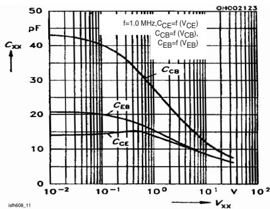
Figure 11. Transistor Capacitance
