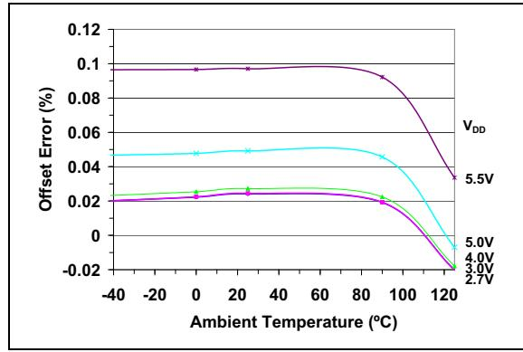
**FIGURE 2-20:** Offset Error vs. Ambient Temperature and  $V_{DD}$ .
