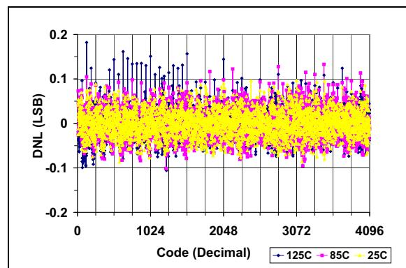
**FIGURE 2-2:** DNL vs. Code and Temperature (MCP4922).
