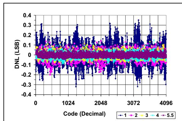
**FIGURE 2-3:** DNL vs. Code and  $V_{REF}$  Gain = 1 (MCP4922).
