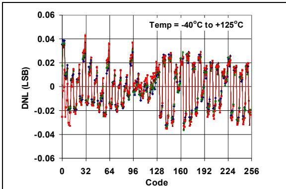
**FIGURE 2-13:** DNL vs. Code and Temperature (MCP4902).
