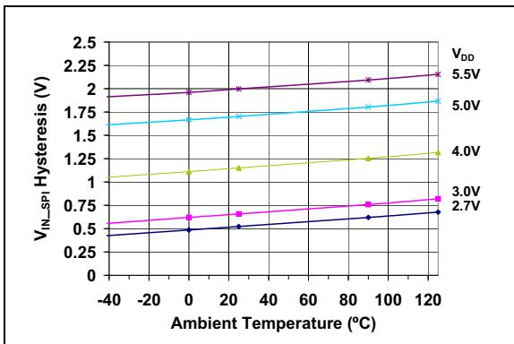
**FIGURE 2-24:** Input Hysteresis vs. Ambient Temperature and  $V_{DD}$ .
