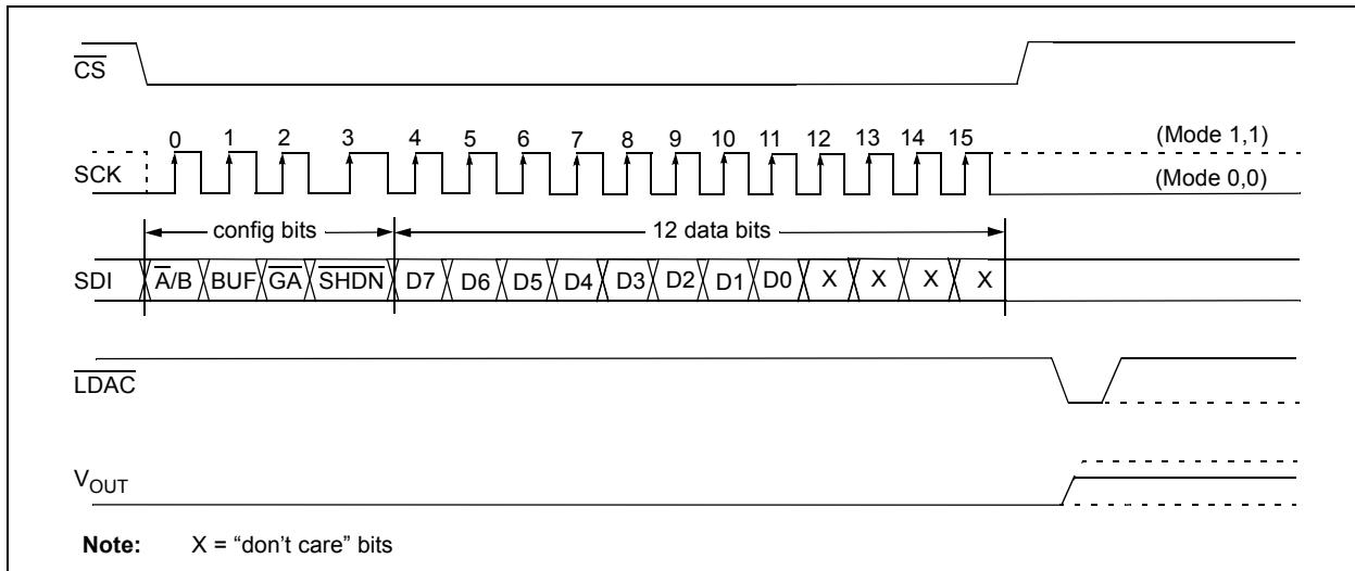
**FIGURE 5-3:** Write Command for MCP4902 (8-bit DAC).
