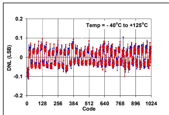
**FIGURE 2-11:** DNL vs. Code and Temperature (MCP4912).
