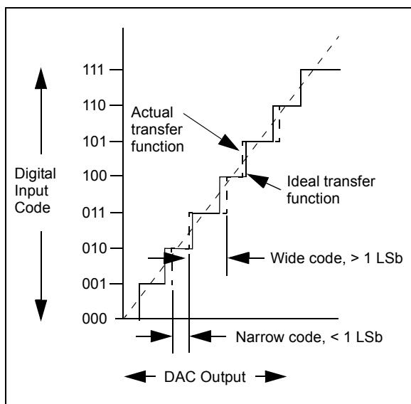
FIGURE 4-2: Example for DNL Accuracy.
