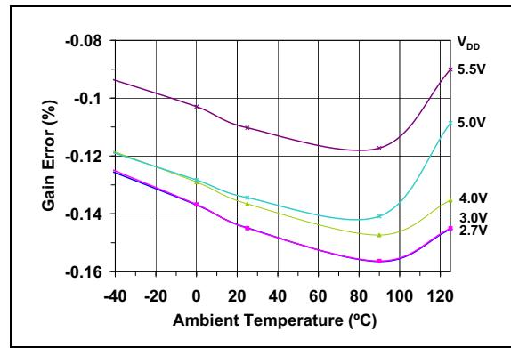
**FIGURE 2-21:** Gain Error vs. Ambient Temperature and  $V_{DD}$ .
