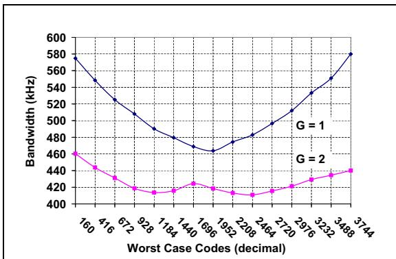
**FIGURE 2-37:** -3 db Bandwidth vs. Worst Codes.
