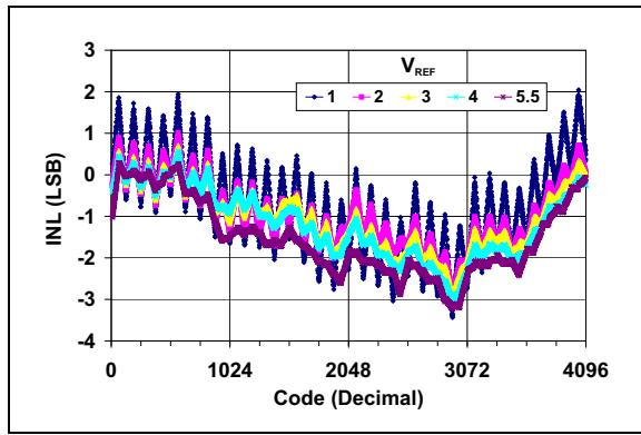
**FIGURE 2-9:** INL vs. Code and  $V_{REF}$  (MCP4922).
