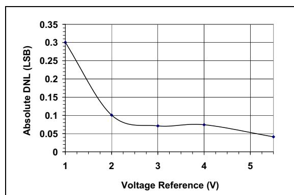
**FIGURE 2-5:** Absolute DNL vs. Voltage Reference (MCP4922).
