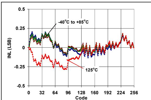
**FIGURE 2-14:** INL vs. Code and Temperature (MCP4902).
