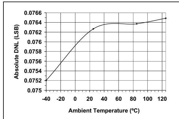
**FIGURE 2-4:** Absolute DNL vs. Temperature (MCP4922).
