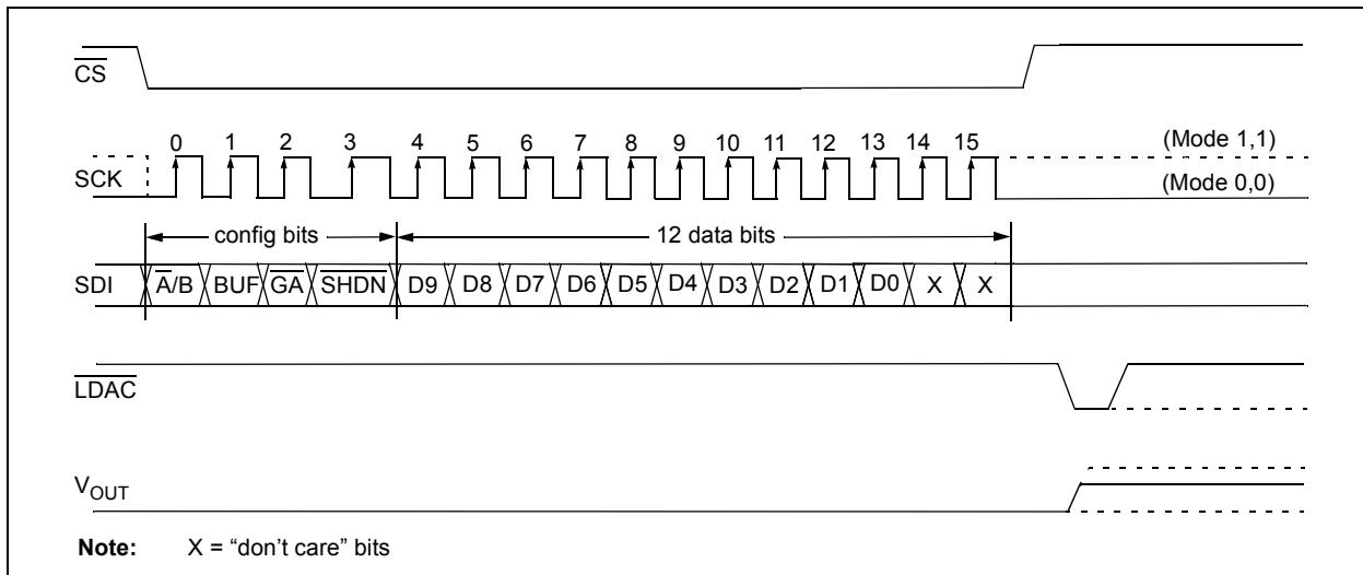
**FIGURE 5-2:** Write Command for MCP4912 (10-bit DAC).
