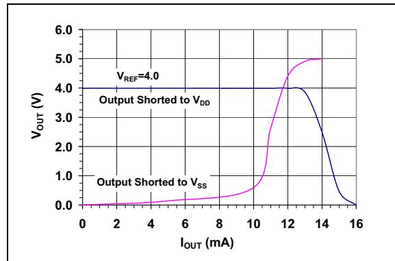
**FIGURE 2-29:**  $I_{OUT}$  vs  $V_{OUT}$ . Gain = 1x.
