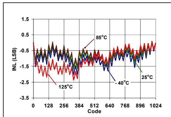
**FIGURE 2-12:** INL vs. Code and Temperature (MCP4912).
