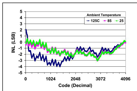
**FIGURE 2-6:** INL vs. Code and Temperature (MCP4922).
