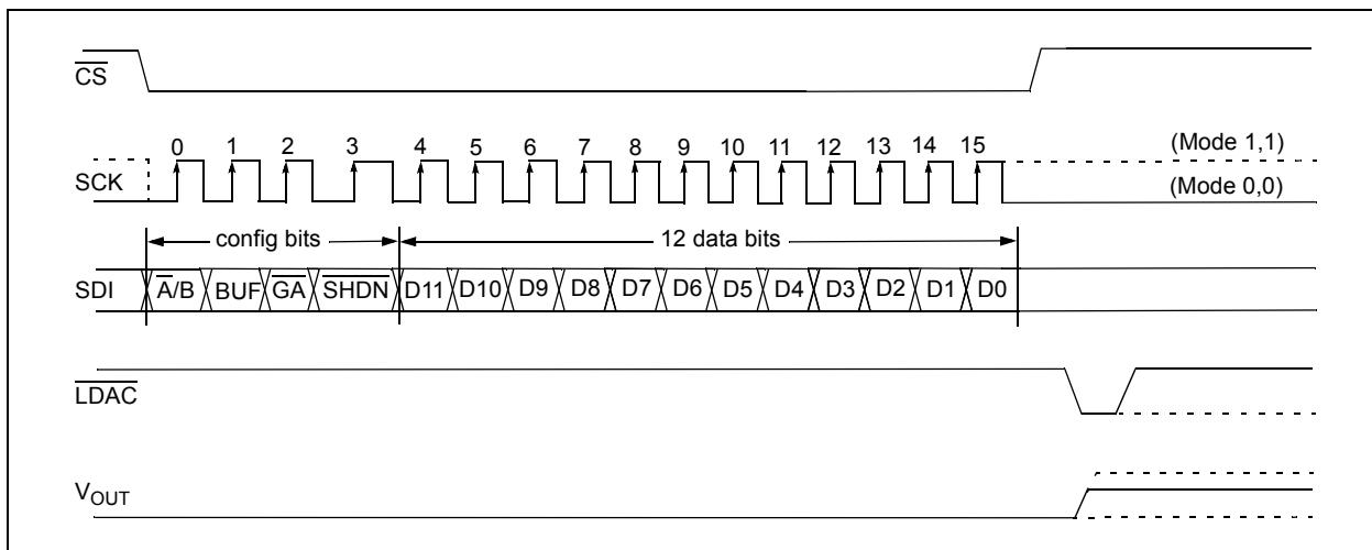
**FIGURE 5-1:** Write Command for MCP4922 (12-bit DAC).
