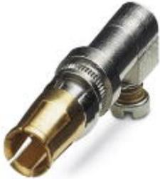
POWER contact, for D-SUB combination inserts, screw connection, socket, straight, rated current 20 A, gold-plated
