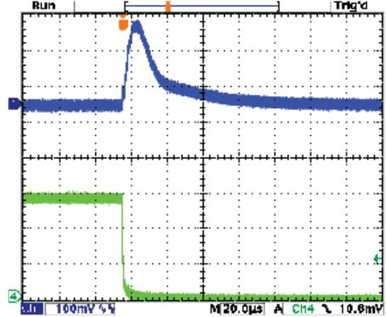
Step Load Transient Response (Vin=7.5V, Vout=5V, Cload=5x10µF X5R 0805 ceramic, total 50µF, Iout=0A to 1.5A) Top trace=Vout, Bottom trace=Iout
