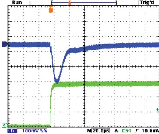
Step Load Transient Response (Vin=12V, Vout=5V, Cload=5x10µF X5R 0805 ceramic, total 50µF, Iout=1.5A to 0A) Top trace=Vout, Bottom trace=Iout
