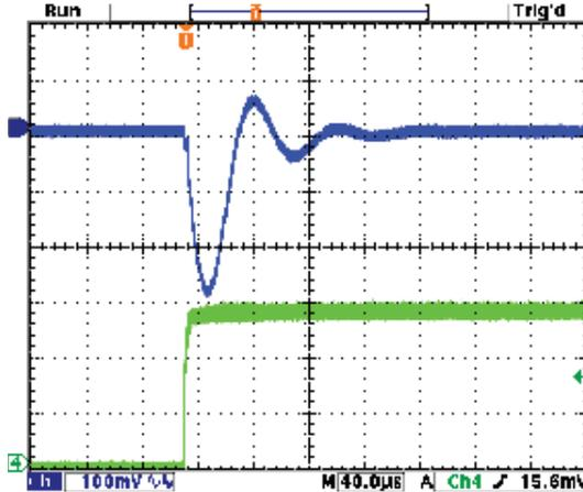
Step Load Transient Response (Vin=4.5V, Vout=1.8V, Cload=5x10µF
