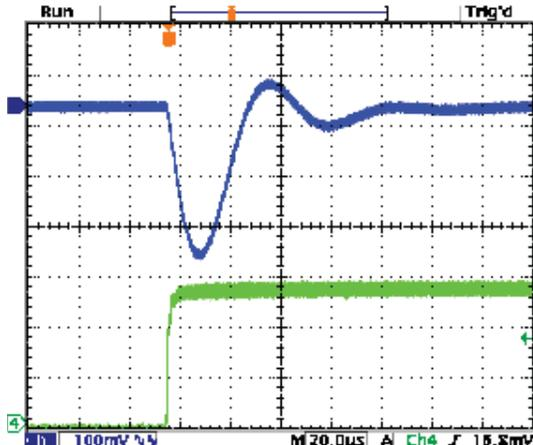
Step Load Transient Response (Vin=5.5V, Vout=3.3V, Cload=5x10µF
