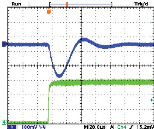
Step Load Transient Response (Vin=7.5V, Vout=5V, Cload=12x10µF X5R 0805 ceramic, total 120µF, Iout=1.5A to 0A) Top trace=Vout, Bottom trace=Iout
