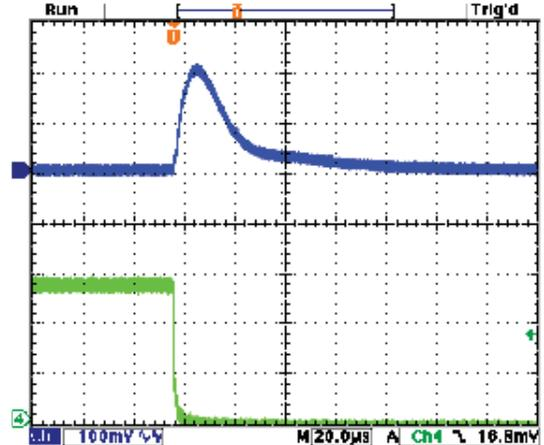
Step Load Transient Response (Vin=4.5V, Vout=1.8V, Cload=5x10µF
