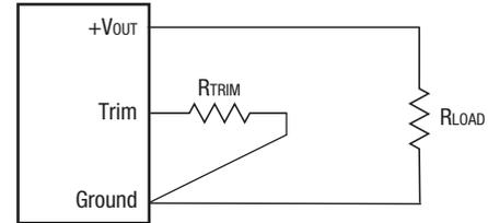
$$R_{TRIM} (k\Omega) = \frac{1.182}{V_{OUT} - 0.591}$$
