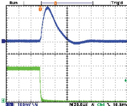
Step Load Transient Response (Vin=12V, Vout=3.3V, Cload=12x10µF
