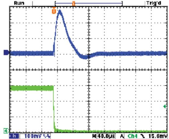
Step Load Transient Response (Vin=12V, Vout=1.8V, Cload=12x10µF
