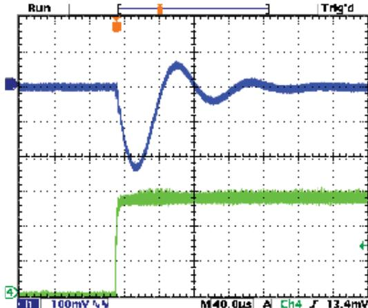
Step Load Transient Response (Vin=5.5V, Vout=3.3V, Cload=12x10µF X5R 0805 ceramic, total 120µF, Iout=1.5A to 0A) Top trace=Vout, Bottom trace=Iout
