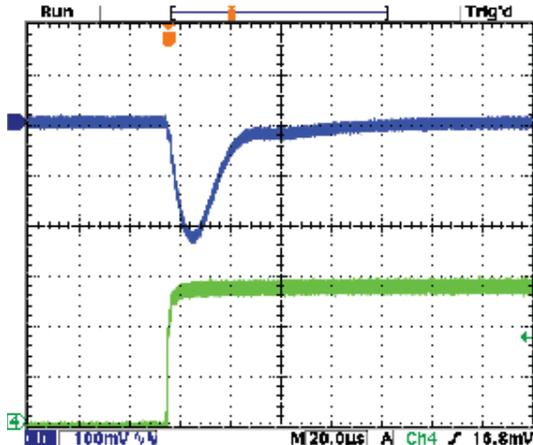
Step Load Transient Response (Vin=12V, Vout=3.3V, Cload=5x10µF
