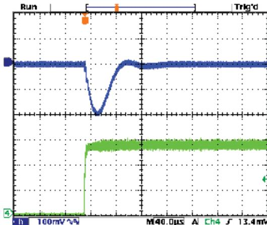
Step Load Transient Response (Vin=12V, Vout=1.8V, Cload=12x10µF
