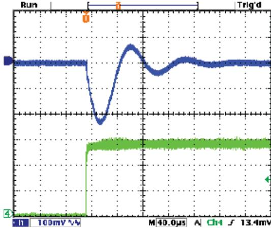
Step Load Transient Response (Vin=4.5V, Vout=1.8V, Load=12x10µF X5R 0805 ceramic, total 120µF, Iout=1.5A to 0A) Top trace=Vout, Bottom trace=Iout
