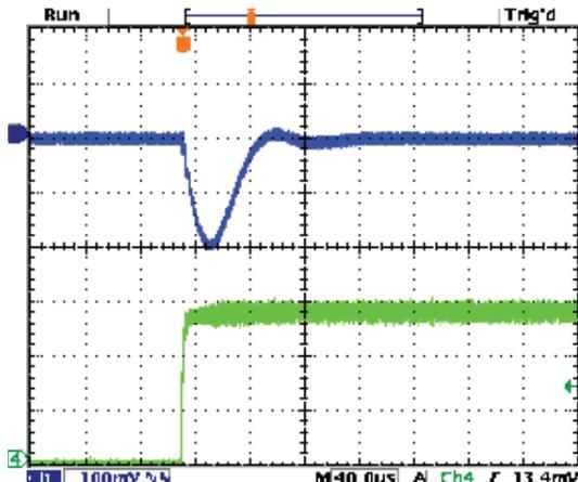
Step Load Transient Response (Vin=12V, Vout=3.3V, Cload=12x10µF
