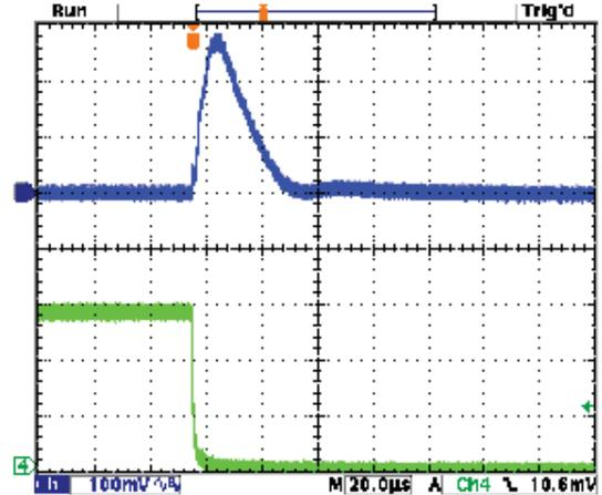
Step Load Transient Response (Vin=12V, Vout=5V, Cload=12x10µF X5R 0805 ceramic, total 120µF, Iout=0A to 1.5A) Top trace=Vout, Bottom trace=Iout
