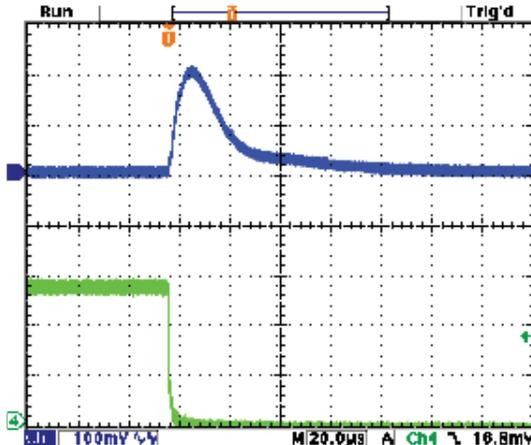
Step Load Transient Response (Vin=5.5V, Vout=3.3V, Cload=5x10µF
