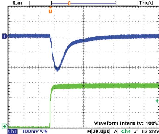
Step Load Transient Response (Vin=12V, Vout=1.8V, Cload=5x10µF
