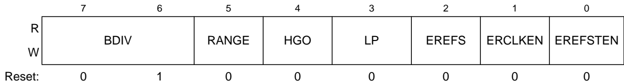
Figure 11-4. ICS Control Register 2 (ICSC2)
