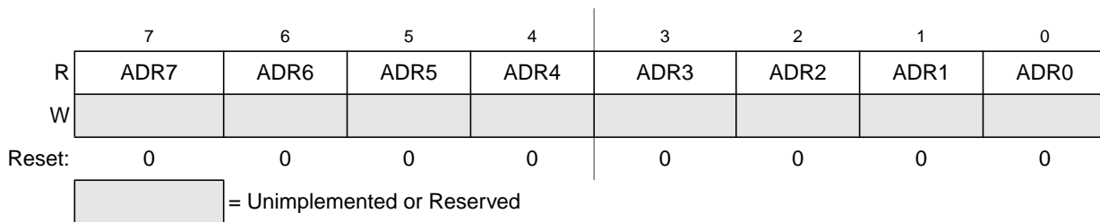
Figure 9-6. Data Result Low Register (ADCRL)
