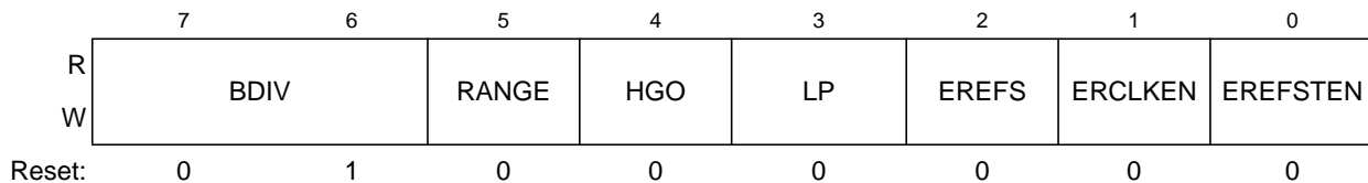
Figure 11-4. ICS Control Register 2 (ICSC2)
