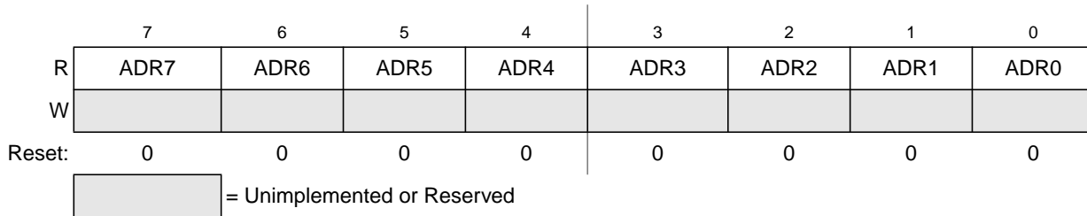
Figure 9-6. Data Result Low Register (ADCRL)
