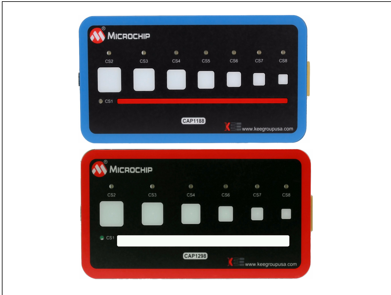
Figure 1.2 CAP1xxx Evaluation Board Top View
