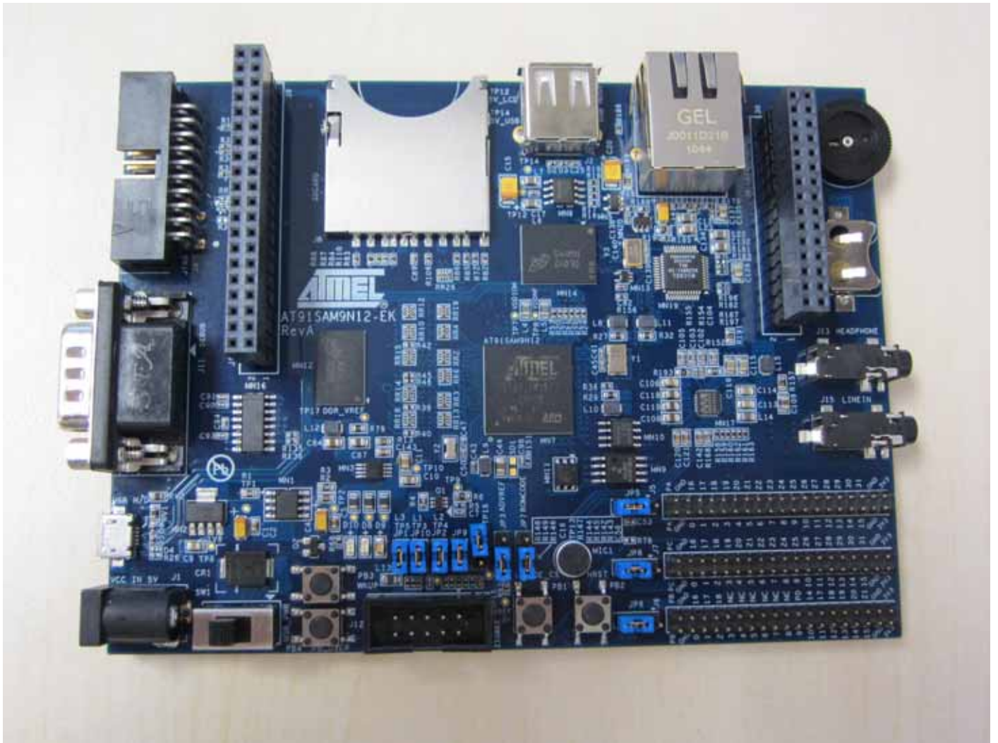
Figure 4-3. SAM9N12-EK Board Layout
