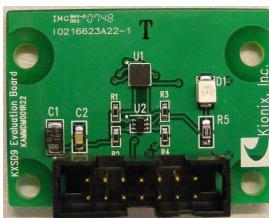
To facilitate prototype work with Kionix accelerometers,
