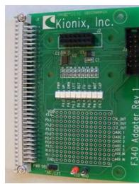
The Kionix F340 Adapter Board provides the link between the accelerometer Evaluation Board and the Silicon Labs C8051F340-TB. Two connectors are provided for connecting Evaluation Boards to the Adapter Board. Evaluation Boards can be plugged in directly or tethered via a ribbon cable. The tethered connection can be useful when evaluating screen rotation, tap/double-tap, or motion wake-up functionality since the accelerometer can be more easily manipulated.
