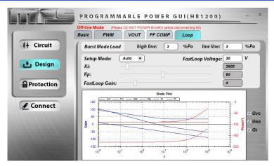
Figure 17: Design-Loop Panel
