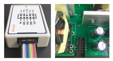
Figure 8: EVB to MPS I<sup>2</sup>C Dongle Wire Connection
