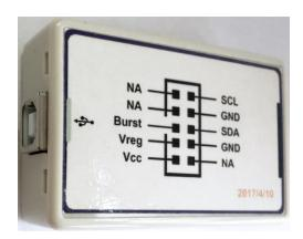
Figure 3: EVHR1200 PMBUS Kit-01A Dongle
