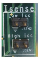
**Figure 5. Current Monitor Sense Points**
