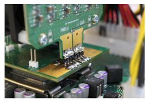
Figure 2. DLT Attached to Interposer with Header Pins
