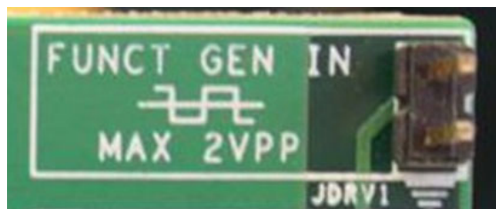
Figure 9. Internal Drive (Square Wave Input)
