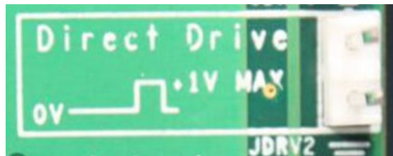
Figure 7. Direct Drive (Drives DLT Load Amps Directly)
