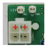
**Figure 6. Input Power Connection**
