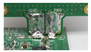
Figure 1. DLT Attached with Solder Wick
