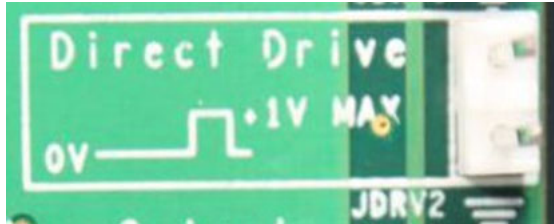
Figure 7. Direct Drive (Drives DLT Load Amps Directly)
