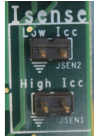
Figure 5. Current Monitor Sense Points
