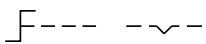
15 Selector switch actuator 3 positions page 24 | Selector switch actuator 3 positions, flush mounting page 36
