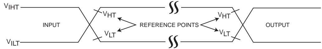
FIGURE 8-5: AC INPUT/OUTPUT REFERENCE WAVEFORMS
