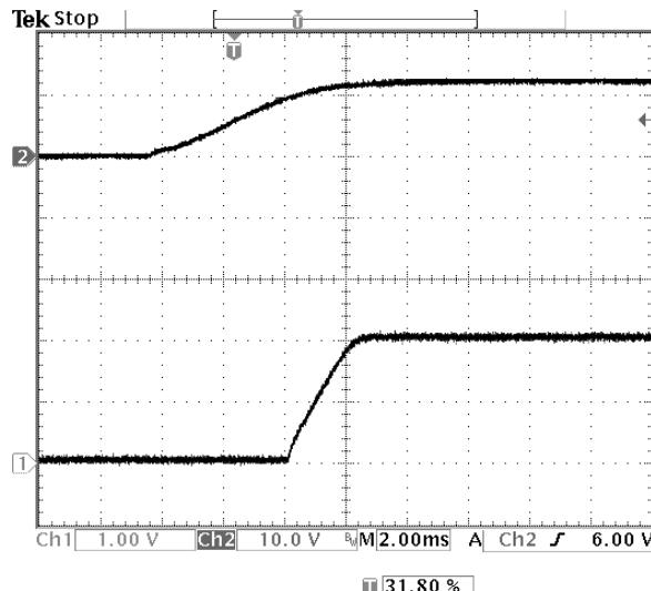
**Fig-2.0V-4:** Turn-on transient for  $V_{out}=2.0V$  with application of  $V_{in}$  at full rated load current (resistive) and  $47\mu Fx2$  external capacitance at  $V_{in}=12V$ .
