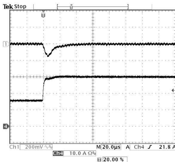
**Fig-2.5V-6:** Output voltage response for  $V_{out}=2.5V$  to positive load current step change from 15A to 30A with slew rate of  $5A/\mu s$  at  $V_{in}=12V$ .  $C_o=47\mu Fx2$  ceramic.
