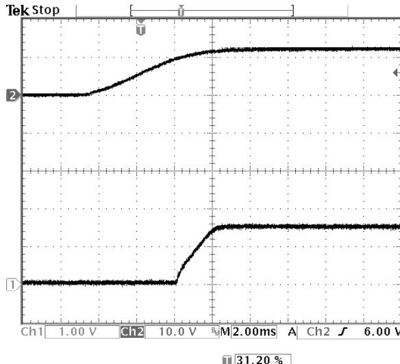
**Fig-1.5V-4:** Turn-on transient for  $V_{out}=1.5V$  with application of  $V_{in}$  at full rated load current (resistive) and  $47\mu Fx2$  external capacitance at  $V_{in}=12V$ .
