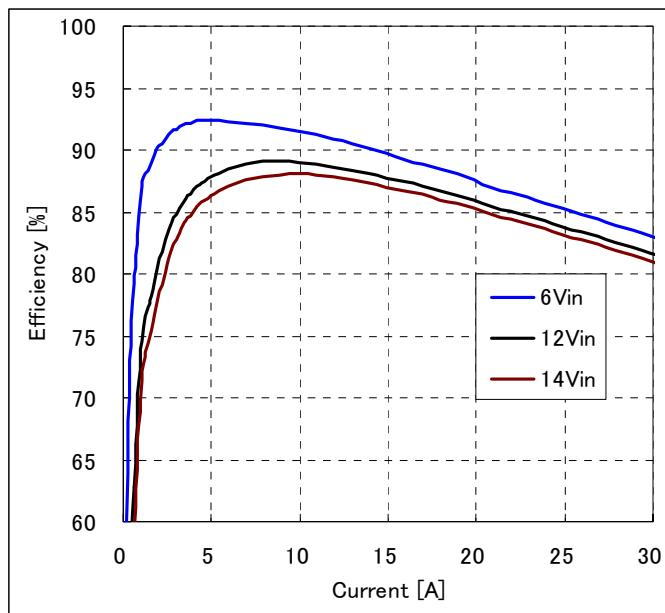
**Fig-1.2V-2:** Efficiency vs. load current and input voltage for  $V_{out}=1.2V$ . Airflow rate=200 LFM (1m/s) and  $T_a=25^{\circ}C$ .
