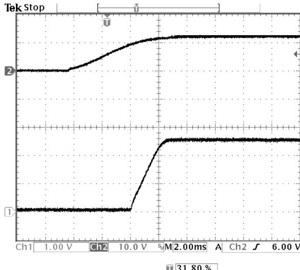
**Fig-2.5V-4:** Turn-on transient for  $V_{out}=2.5V$  with application of  $V_{in}$  at full rated load current (resistive) and  $47\mu Fx2$  external capacitance at  $V_{in}=12V$ .
