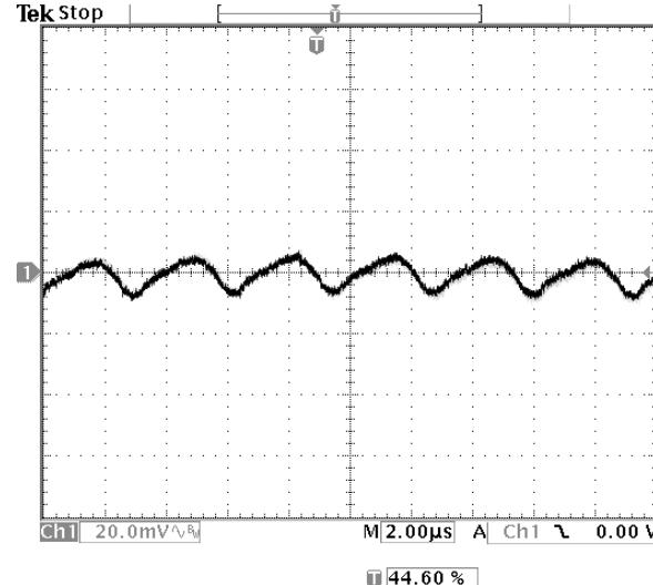
**Fig-2.5V-5:** Output voltage ripple (20mV/div.) for  $V_{out}=2.5V$  at full rated load current into a resistive load with external capacitance  $47\mu Fx2$  ceramic +  $1\mu F$  ceramic at  $V_{in}=12V$ .
