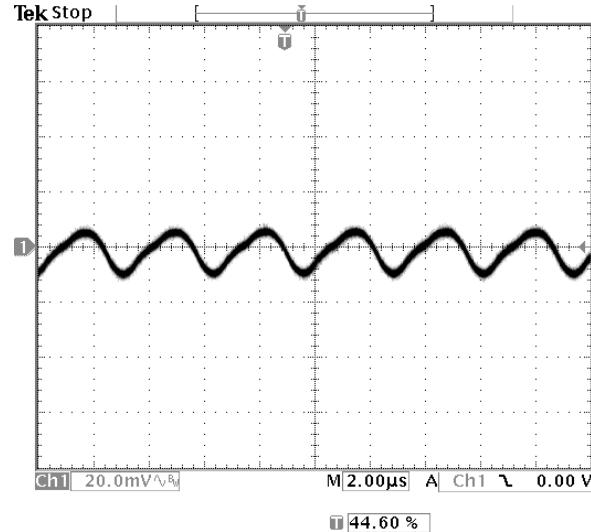
**Fig-3.3V-6:** Output voltage response for  $V_{out}=3.3V$  to positive load current step-change from 15A to 30A with slew rate of 5A/us at  $V_{in}=12V$ .  $C_o=47\mu Fx2$  ceramic.
