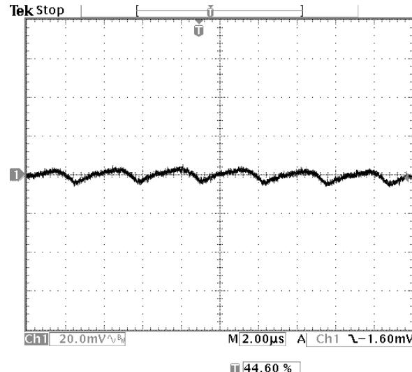
**Fig-1.5V-5:** Output voltage ripple (20mV/div.) for  $V_{out}=1.5V$  at full rated load current into a resistive load with external capacitance  $47\mu Fx2$  ceramic +  $1\mu F$  ceramic at  $V_{in}=12.0V$ .
