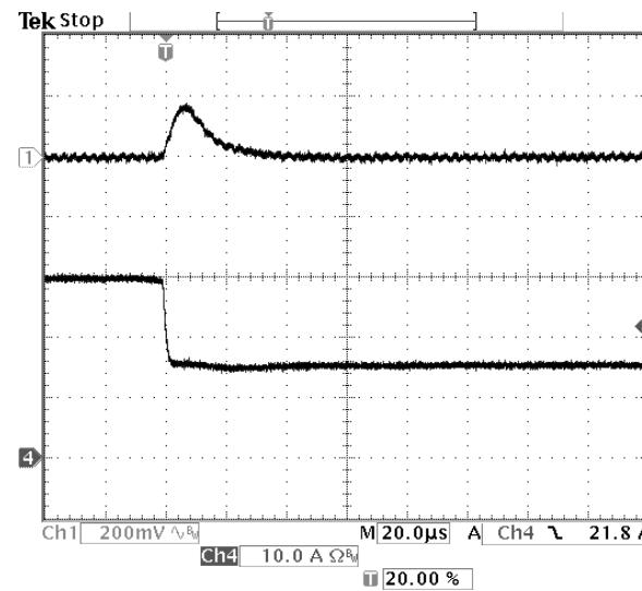
**Fig-2.5V-7:** Output voltage response for  $V_{out}=2.5V$  to negative load current step change from 30A to 15A with slew rate of  $-5A/\mu s$  at  $V_{in}=12V$ .  $C_o=47\mu Fx2$  ceramic.
