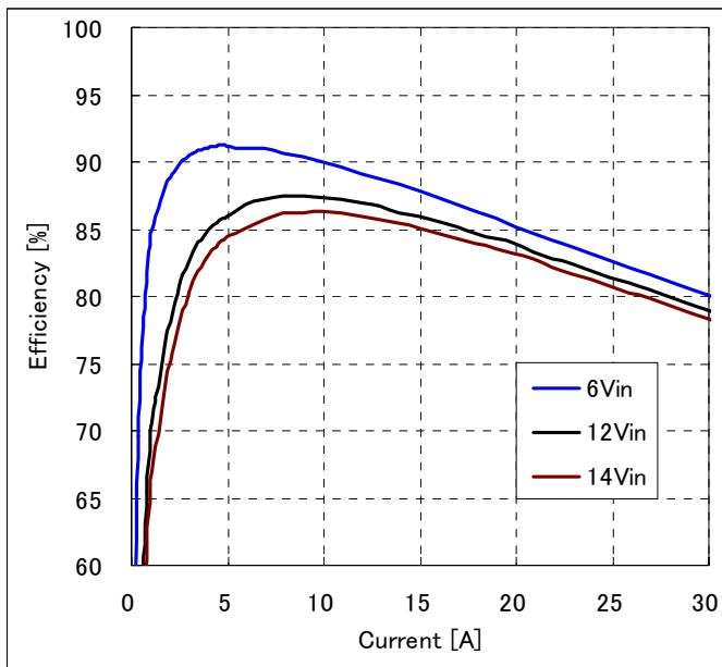
**Fig-1.0V-2:** Efficiency vs. load current and input voltage for  $V_{out}=1.0V$ . Airflow rate=200 LFM (1m/s) and  $T_a=25^{\circ}C$ .
