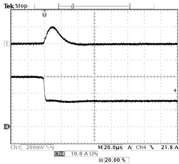
**Fig-1.0V-7:** Output voltage response for  $V_{out}=1.0V$  to negative load current step change from 30A to 15A with slew rate of  $-5A/\mu s$  at  $V_{in}=12V$ .  $C_o=47\mu Fx2$  ceramic.
