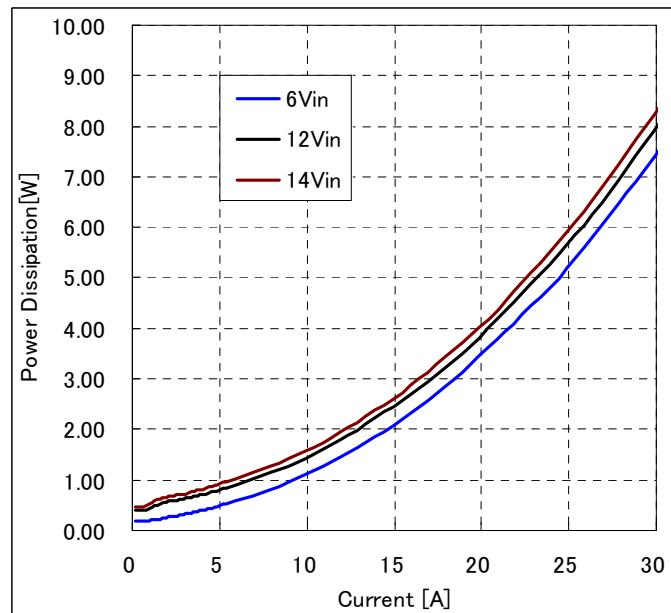
**Fig-1.0V-3:** Power Loss vs. load current and input voltage for  $V_{out}=1.0V$ . Airflow rate=200 LFM (1m/s) and  $T_a=25^{\circ}C$ .
