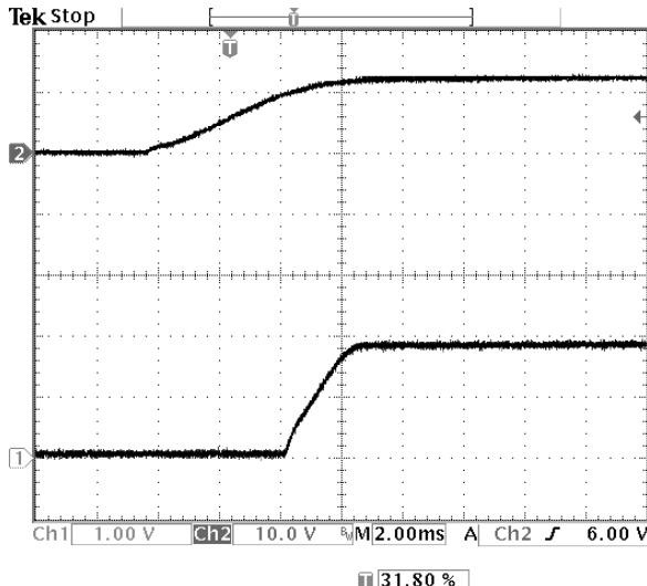
**Fig-1.8V-4:** Turn-on transient for  $V_{out}=1.8V$  with application of  $V_{in}$  at full rated load current (resistive) and  $47\mu Fx2$  external capacitance at  $V_{in}=12V$ .
