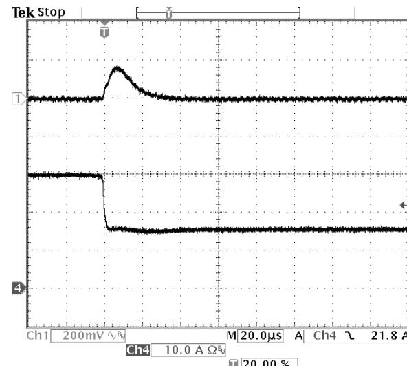
**Fig-1.8V-7:** Output voltage response for  $V_{out}=1.8V$  to negative load current step change from 30A to 15A with slew rate of  $-5A/\mu s$  at  $V_{in}=12V$ .  $C_o=47\mu Fx2$  ceramic.
