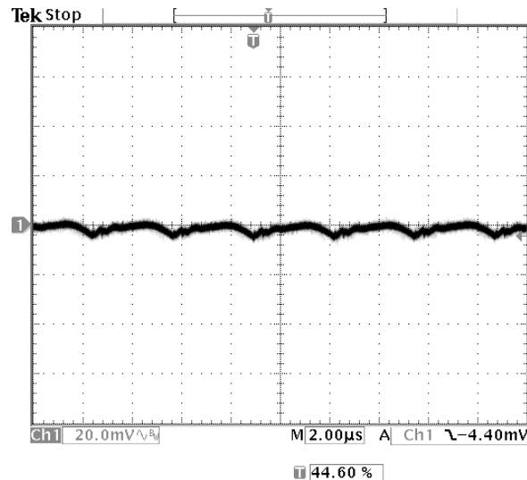
**Fig-1.0V-5:** Output voltage ripple (20mV/div.) for  $V_{out}=1.0V$  at full rated load current into a resistive load with external capacitance  $47\mu Fx2$  ceramic +  $1\mu F$  ceramic at  $V_{in}=12V$ .
