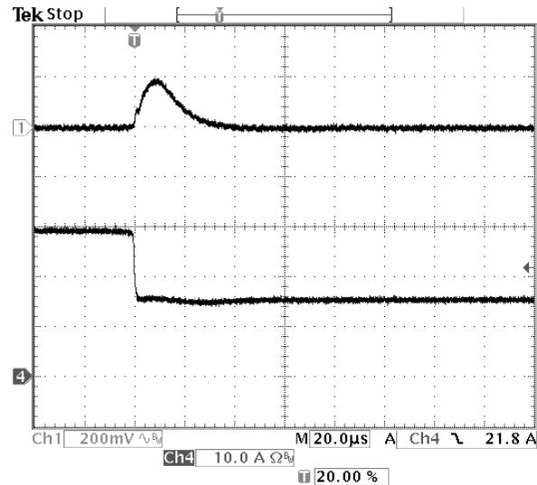
**Fig-1.2V-8:** Output voltage response for  $V_{out}=1.2V$  to negative load current step change from 30A to 15A with slew rate of -5A/us at  $V_{in}=12V$ .  $C_o=47\mu Fx2$  ceramic.
