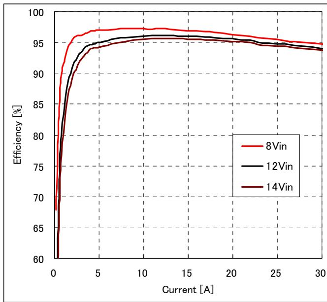
**Fig-5.0V-2:** Efficiency vs. load current and input voltage for  $V_{out}=5.0V$ .
