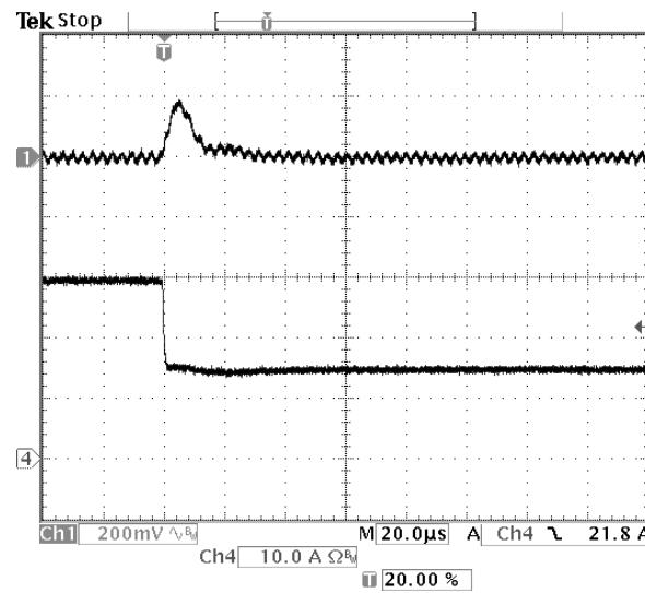
Fig-5.0V-6: Output voltage response for  $V_{out}=5.0V$  to positive load current step change from 15A to 30A with slew rate of  $5A/\mu s$  at  $V_{in}=12V$ .  $C_o=47\mu Fx2$  ceramic.
