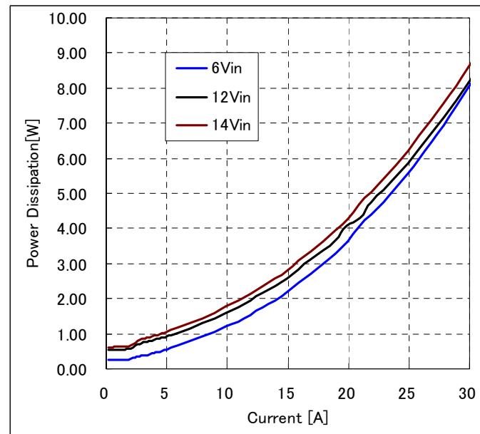
**Fig-2.0V-3:** Power Loss vs. load current and input voltage for  $V_{out}=2.0V$ .
