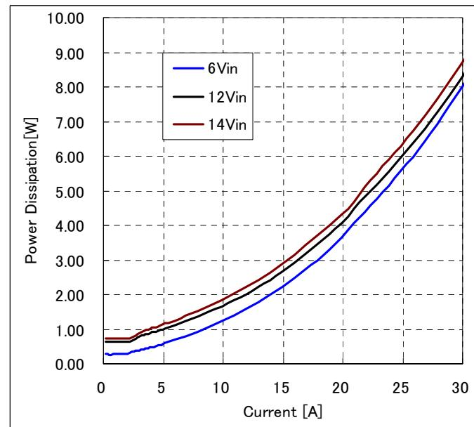
**Fig-2.5V-3:** Power Loss vs. load current and input voltage for  $V_{out}=2.5V$ . Airflow rate=200 LFM (1m/s) and  $T_a=25^{\circ}C$ .
