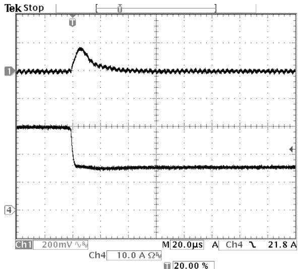
**Fig-3.3V-8:** Output voltage response for  $V_{out}=3.3V$  to negative load current step change from 30A to 15A with slew rate of -5A/us at  $V_{in}=12V$ .  $C_o=47\mu Fx2$  ceramic.
