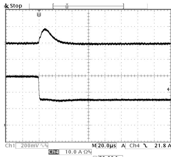
**Fig-1.5V-7:** Output voltage response for  $V_{out}=1.5V$  to negative load current step change from 30A to 15A with slew rate of  $-5A/\mu s$  at  $V_{in}=12V$ .  $C_o=47\mu Fx2$  ceramic.
