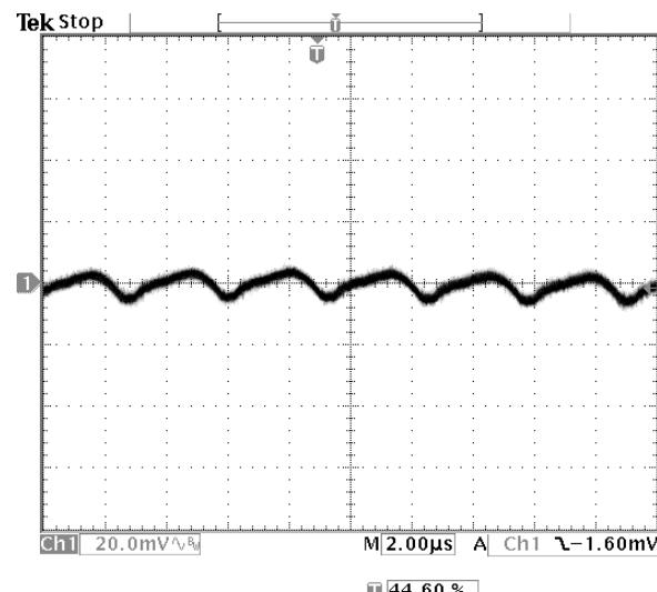
**Fig-2.0V-5:** Output voltage ripple (20mV/div.) for  $V_{out}=2.0V$  at full rated load current into a resistive load with external capacitance  $47\mu Fx2$  ceramic +  $1\mu F$  ceramic at  $V_{in}=12V$ .
