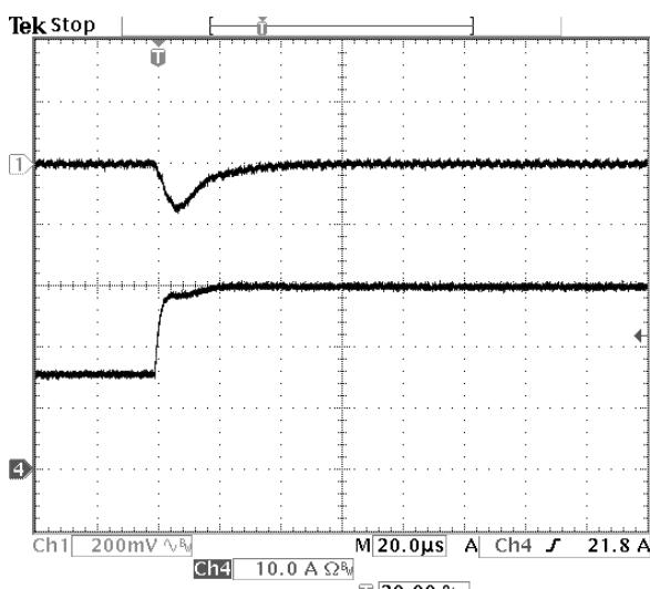
**Fig-1.8V-6:** Output voltage response for  $V_{out}=1.8V$  to positive load current step change from 15A to 30A with slew rate of  $5A/\mu s$  at  $V_{in}=12V$ .  $C_o=47\mu Fx2$  ceramic.
