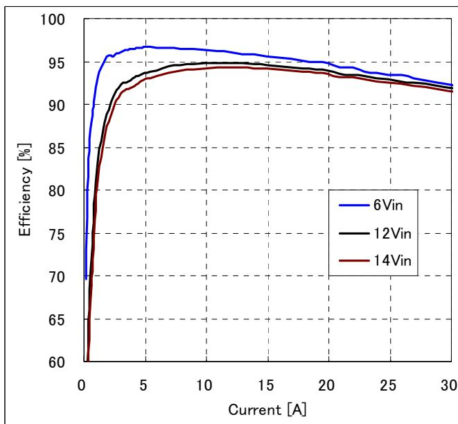
**Fig-3.3V-2:** Efficiency vs. load current and input voltage for  $V_{out}=3.3V$ . Airflow rate=200 LFM (1m/s) and  $T_a=25^{\circ}C$ .
