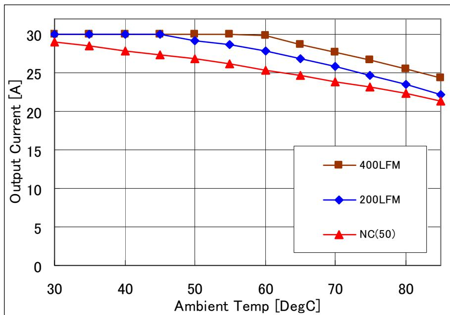
**Fig-1.0V-1:** Available load current vs. ambient temperature and airflow rates for  $V_{out}=1.0V$  with  $V_{in}=12V$ . Maximum component temperature  $\leq 120^{\circ}C$
