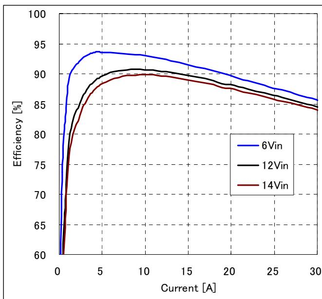
**Fig-1.5V-2:** Efficiency vs. load current and input voltage for  $V_{out}=1.5V$ . Airflow rate=200 LFM (1m/s) and  $T_a=25^{\circ}C$ .
