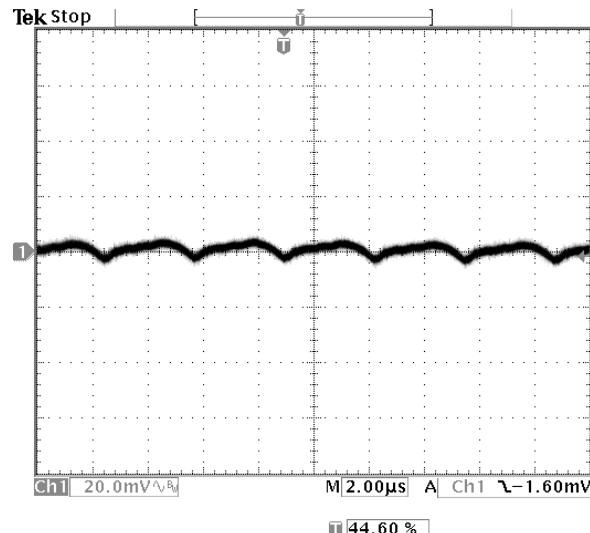
**Fig-1.2V-6:** Output voltage response for  $V_{out}=1.2V$  to positive load current step change from 15A to 30A with slew rate of 5A/us at  $V_{in}=12V$ .  $C_o=47\mu Fx2$  ceramic.
