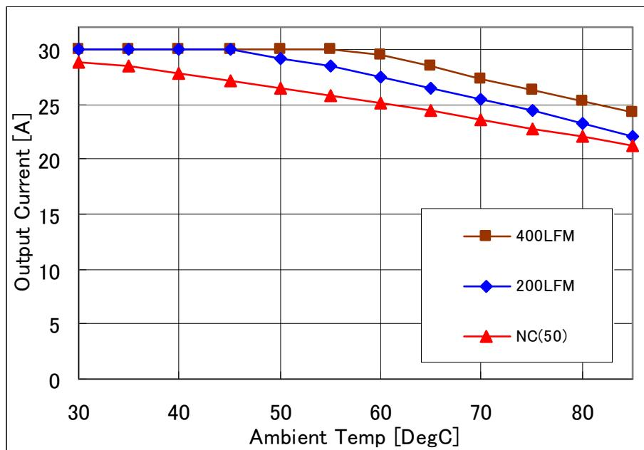
**Fig-1.2V-1:** Available load current vs. ambient temperature and airflow rates for  $V_{out}=1.2V$  with  $V_{in}=12V$ . Maximum component temperature  $\leq 120^{\circ}C$
