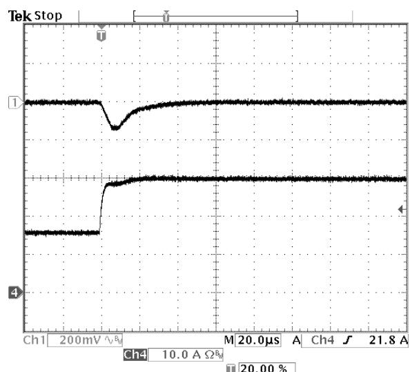
**Fig-2.0V-6:** Output voltage response for  $V_{out}=2.0V$  to positive load current step change from 15A to 30A with slew rate of  $5A/\mu s$  at  $V_{in}=12V$ .  $C_o=47\mu Fx2$  ceramic.
