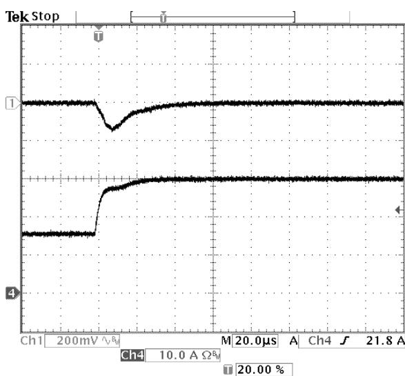
**Fig-1.0V-6:** Output voltage response for  $V_{out}=1.0V$  to positive load current step change from 15A to 30A with slew rate of  $5A/\mu s$  at  $V_{in}=12V$ .  $C_o=47\mu Fx2$  ceramic.
