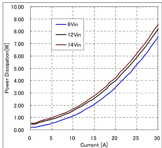
**Fig-1.5V-3:** Power Loss vs. load current and input voltage for  $V_{out}=1.5V$ . Airflow rate=200 LFM (1m/s) and  $T_a=25^{\circ}C$ .
