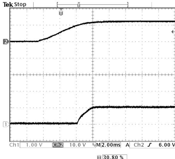
**Fig-1.0V-4:** Turn-on transient for  $V_{out}=1.0V$  with application of  $V_{in}$  at full rated load current (resistive) and  $47\mu Fx2$  external capacitance at  $V_{in}=12V$ .
