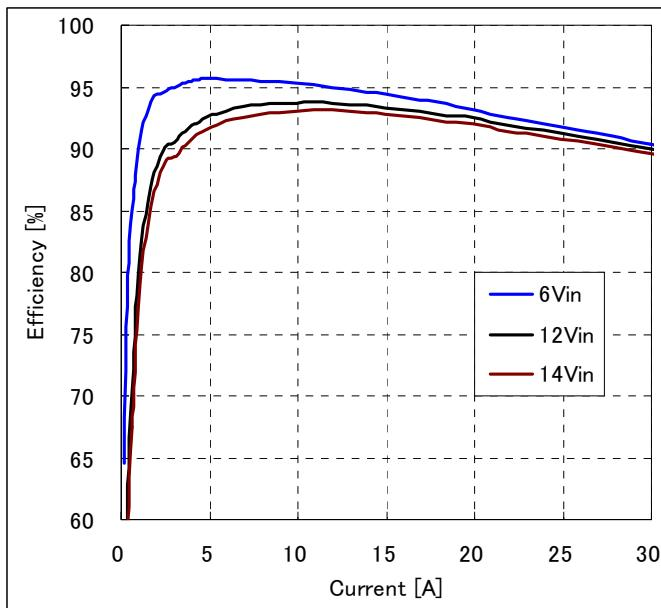
**Fig-2.5V-2:** Efficiency vs. load current and input voltage for  $V_{out}=2.5V$ . Airflow rate=200 LFM (1m/s) and  $T_a=25^{\circ}C$ .
