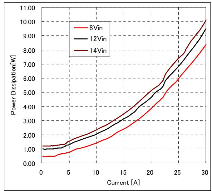
**Fig-5.0V-3:** Power Loss vs. load current and input voltage for  $V_{out}=5.0V$ .
