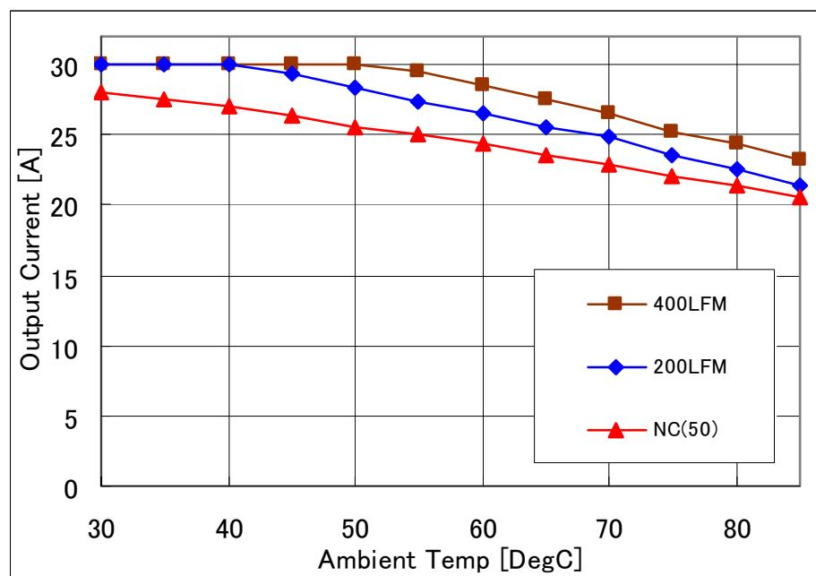
**Fig-2.5V-1:** Available load current vs. ambient temperature and airflow rates for  $V_{out}=2.5V$  with  $V_{in}=12V$ . Maximum component temperature  $\leq 120^{\circ}C$
