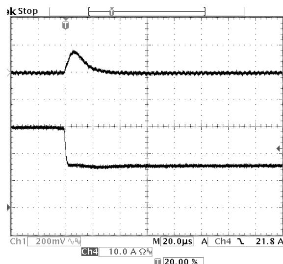
**Fig-2.0V-7:** Output voltage response for  $V_{out}=2.0V$  to negative load current step change from 30A to 15A with slew rate of  $-5A/\mu s$  at  $V_{in}=12V$ .  $C_o=47\mu Fx2$  ceramic.
