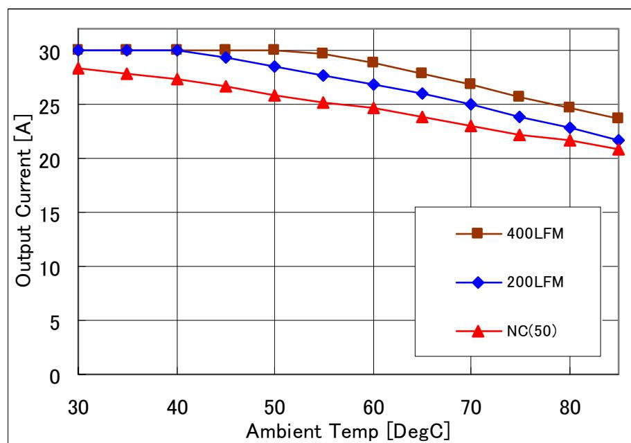
**Fig-2.0V-1:** Available load current vs. ambient temperature and airflow rates for  $V_{out}=2.0V$  with  $V_{in}=12V$ . Maximum component temperature  $\leq 120^{\circ}C$
