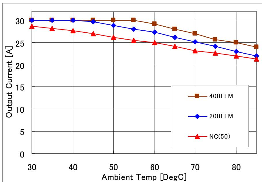
**Fig-1.5V-1:** Available load current vs. ambient temperature and airflow rates for  $V_{out}=1.5V$  with  $V_{in}=12V$ . Maximum component temperature  $\leq 120^{\circ}C$
