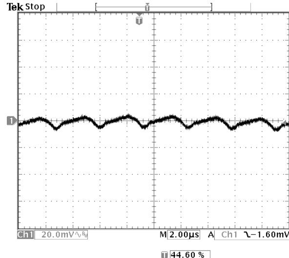
**Fig-1.8V-5:** Output voltage ripple (20mV/div.) for  $V_{out}=1.8V$  at full rated load current into a resistive load with external capacitance  $47\mu Fx2$  ceramic +  $1\mu F$  ceramic at  $V_{in}=12V$ .
