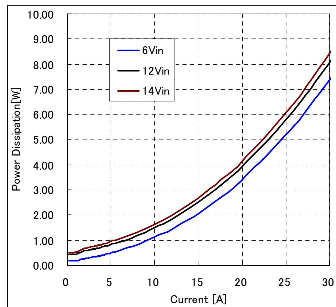
**Fig-1.2V-3:** Power Loss vs. load current and input voltage for  $V_{out}=1.2V$ . Airflow rate=200 LFM (1m/s) and  $T_a=25^{\circ}C$ .
