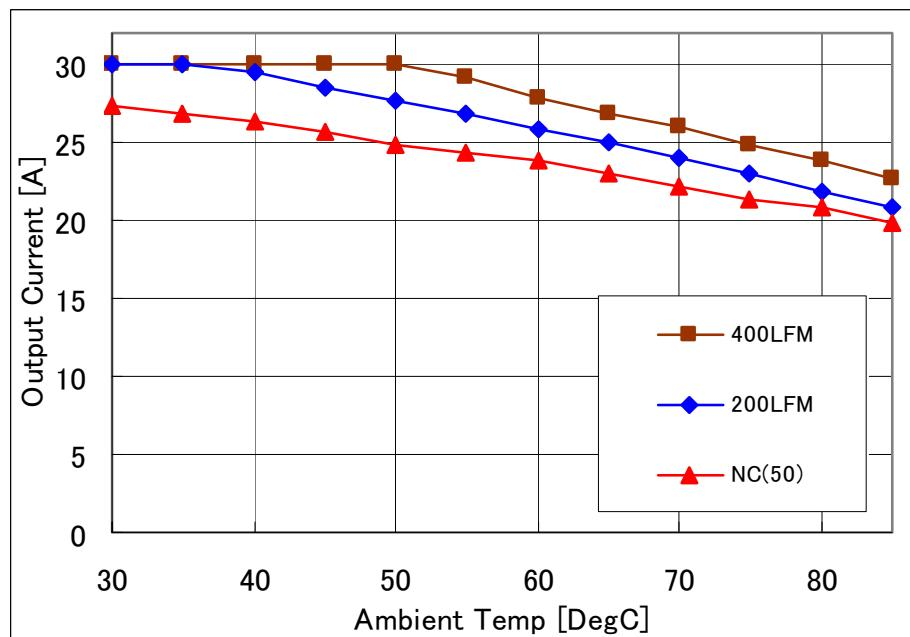
**Fig-3.3V-1:** Available load current vs. ambient temperature and airflow rates for  $V_{out}=3.3V$  with  $V_{in}=12V$ . Maximum component temperature  $\leq 120^{\circ}C$ .
