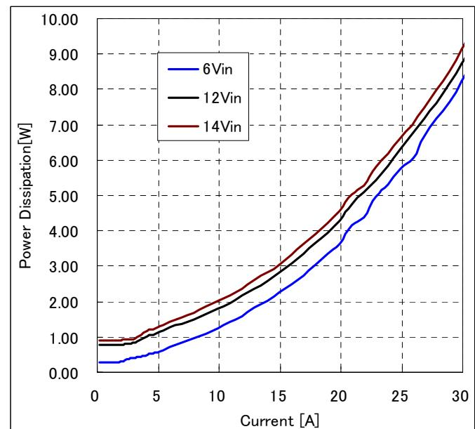
**Fig-3.3V-3:** Power Loss vs. load current and input voltage for  $V_{out}=3.3V$ . Airflow rate=200 LFM (1m/s) and  $T_a=25^{\circ}C$ .
