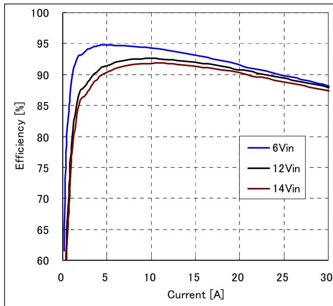
**Fig-2.0V-2:** Efficiency vs. load current and input voltage for  $V_{out}=2.0V$ .
