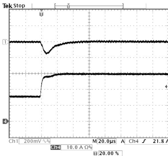
**Fig-1.5V-6:** Output voltage response for  $V_{out}=1.5V$  to positive load current step change from 15A to 30A with slew rate of  $5A/\mu s$  at  $V_{in}=12V$ .  $C_o=47\mu Fx2$  ceramic.
