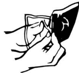
Thoroughly mix by squeezing Compound back and forth 30 to 40 times. Strip Compound from corners while mixing.
