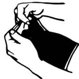
11. Snip off corner of "Unipak" container and pour Compound into Barrel (through opening for inline splice, through upper end for butt splice) until completely full.
