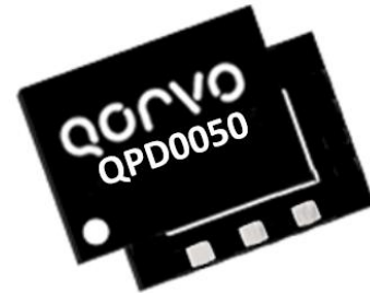
6 Pin 6.6 x 7.7 mm DFN Package
