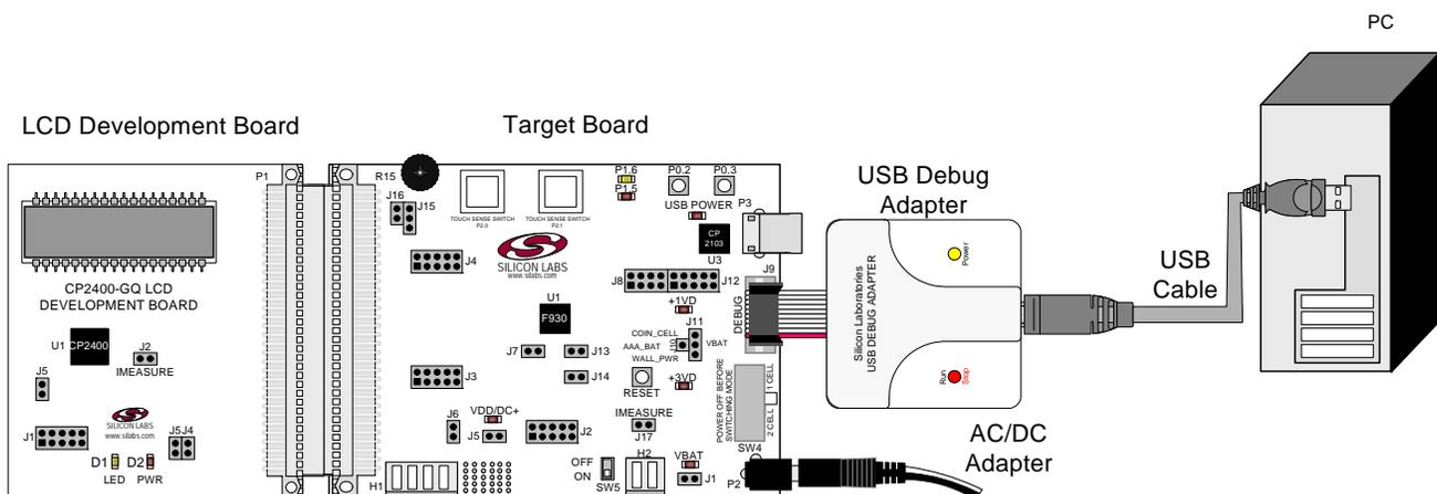
Figure 9. Hardware Setup Using a USB Debug Adapter
