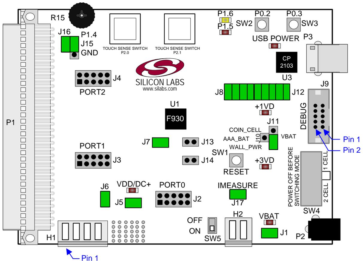
Figure 12. C8051F930 Target Board Shorting Blocks: Factory Defaults
