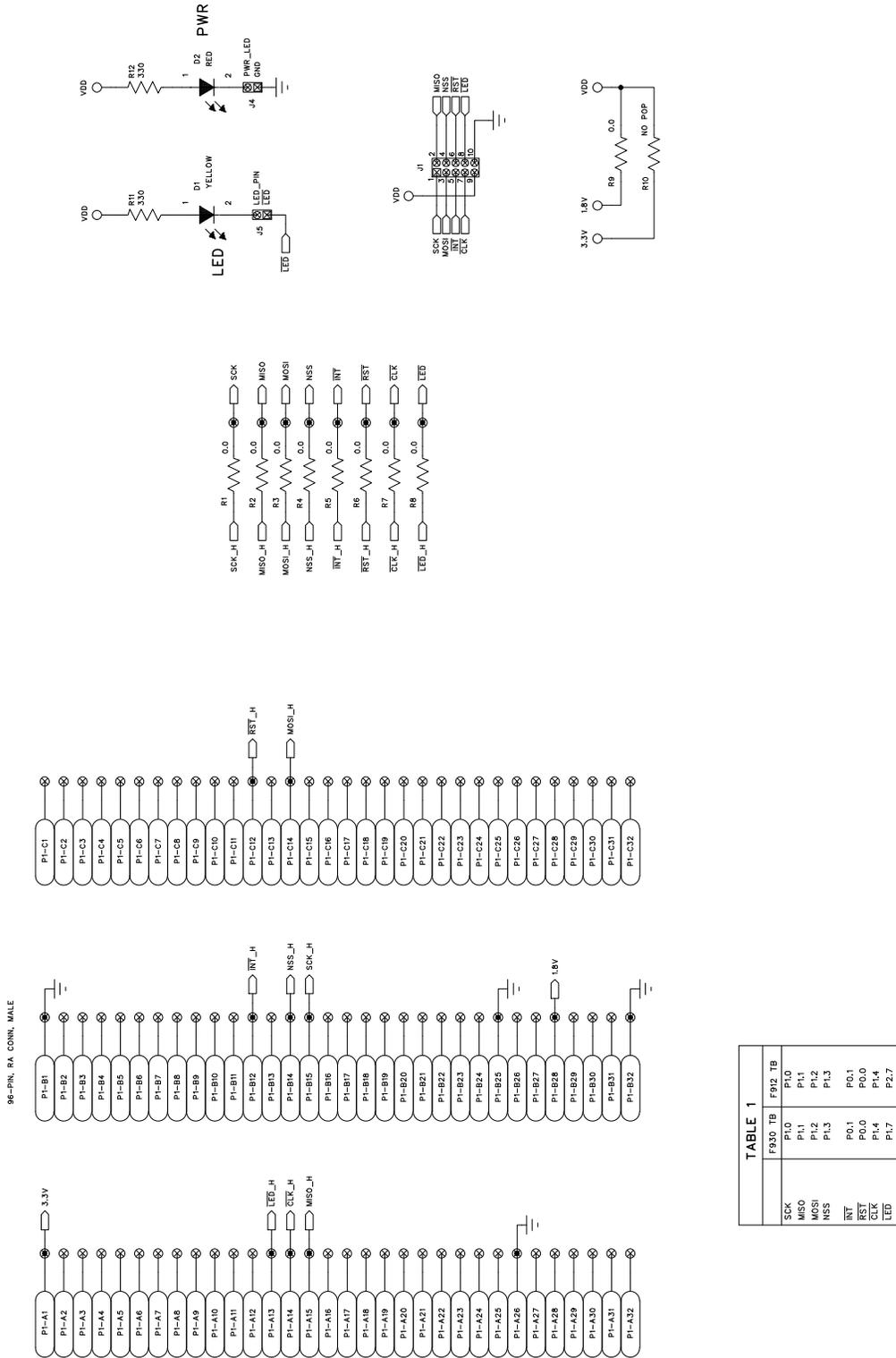
Figure 15. CP2400 LCD Development Board Schematic (Page 1 of 2)
