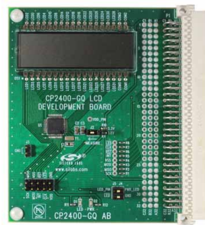
Figure 3. CP2400 Development Board
