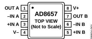
Figure 1. AD8657 Pin Configuration, 8-Lead MSOP
