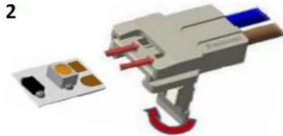
**2** - Insert LED flex ribbon, paying attention to ensure same polarity with wires. Notice that the LED should be aligned with the notched area of the connector and connector latch is on the bottom.
