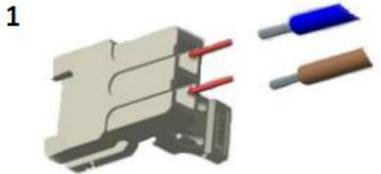
**1** - Insert stripped & tinned wires (20-22 AWG) into cavities. Be sure to push in as far as possible. Gently pull back on wires to ensure that wires are locked into place.
