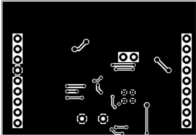
Figure 4-4. Atmel® ATA6628/ATA6630 Development Board; Bottom Side, Top View (as if PCB was Transparent)
