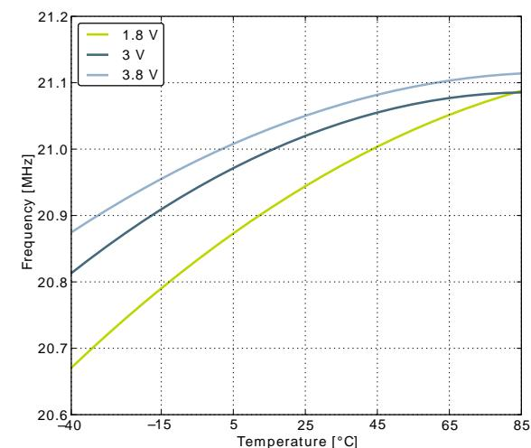
**Figure 3.25. Calibrated HFRCO 28 MHz Band Frequency vs Temperature and Supply Voltage**
