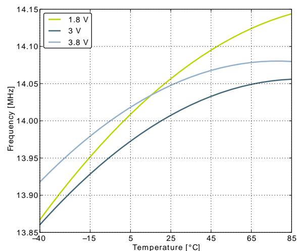
**Figure 3.24. Calibrated HFRCO 21 MHz Band Frequency vs Temperature and Supply Voltage**
