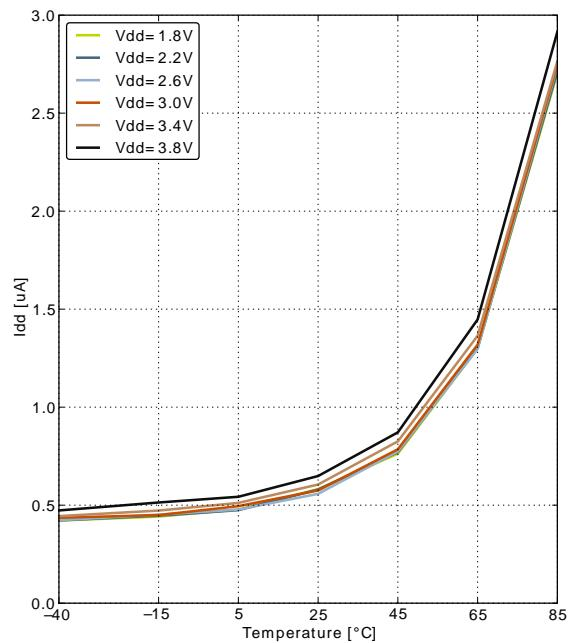
**Figure 3.13. EM4 current consumption.**
