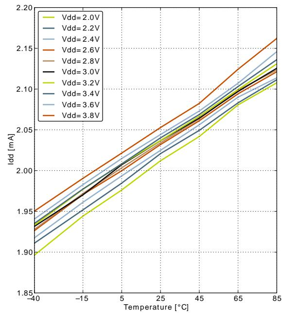
**Figure 3.5. EM0 Current consumption while executing prime number calculation code from flash with HFRCO running at 6.6MHz**
