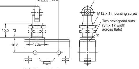
**Note:** Do not use both the M12 mounting screw and the mounting holes in the case at the same time. Doing so will cause stress to be applied to the Switch, possibly damaging the case or cover.
