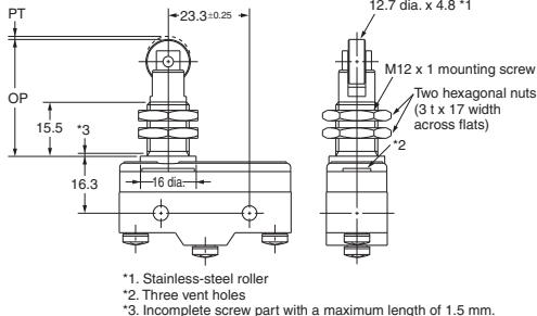
**Note:** Do not use both the M12 mounting screw and the mounting holes in the case at the same time. Doing so will cause stress to be applied to the Switch, possibly damaging the case or cover.
